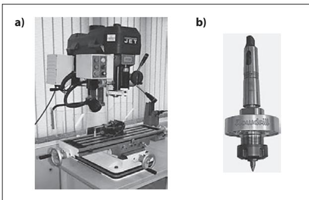
**Figure 2** Milling and drilling center JET JMD-18V (a), Flowdrill tool (b)
