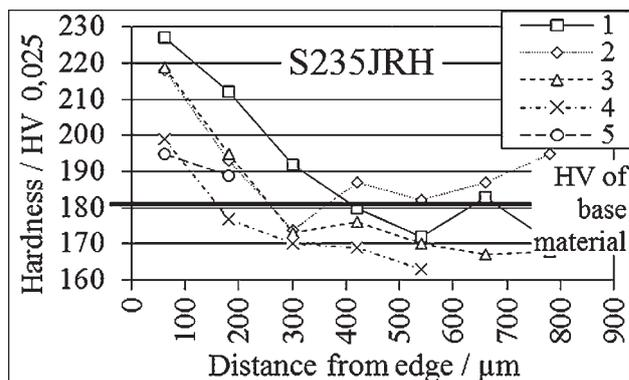
Figure 7 Microhardness of a shape in function of distance from the edge – S235JRH material
