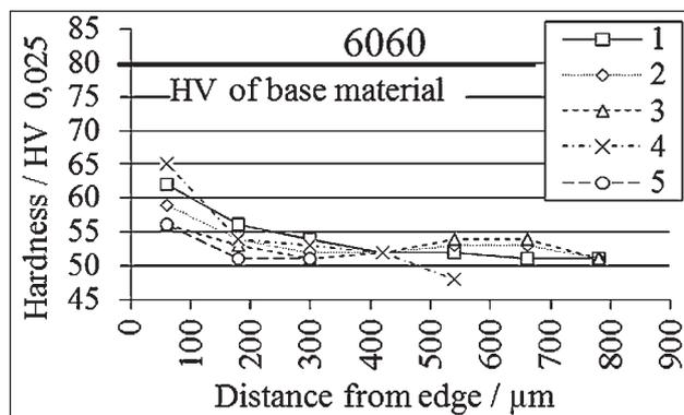
**Figure 9** Microhardness of a shape in function of distance from the edge – 6060 material
