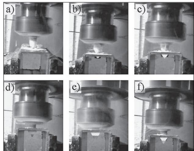
**Figure 1** Flowdrill stages: a) contact of the tool and the material; process after: b) 2 seconds, c) 3 seconds, d) 5 seconds, e) 6 seconds, f) tool retraction [own study]
