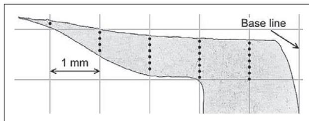
**Figure 4** Locations of measurement of sample microhardness - marked with dots
