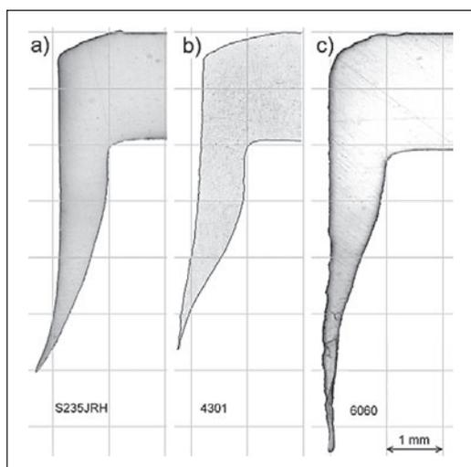
Figure 5 Section of rim of a hole in material: a) S235JRH, b) 4301, c) 6060
