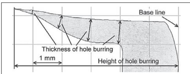
**Figure 3** Scheme of measurement of height and thickness of hole burring
