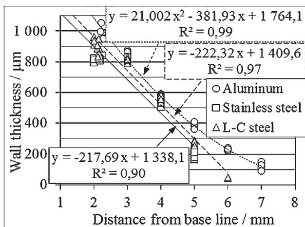
Figure 6 Wall thickness of burred holes in function of height
