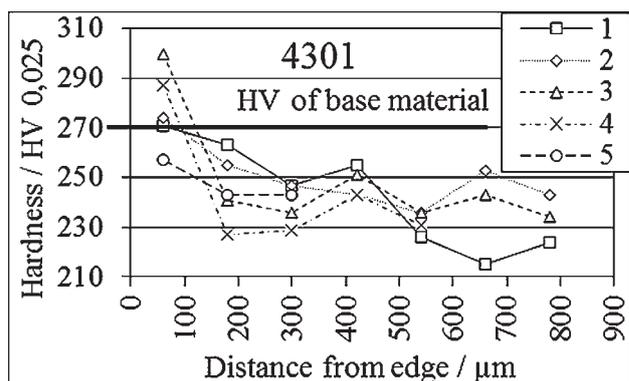
Figure 8 Microhardness of a shape in function of distance from the edge – 4301 material
