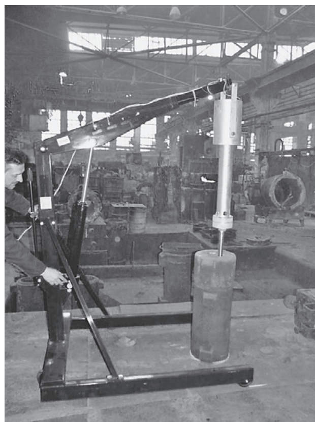
Figure 1 Liquid steel acoustic treatment station
