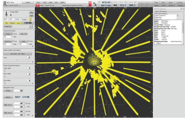
3. d. Amplitude modulated interference 4
