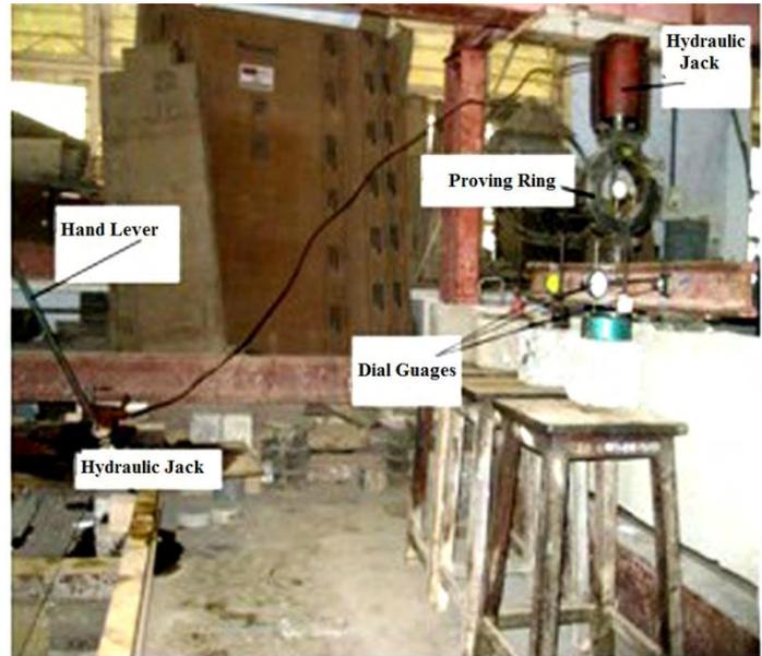
Figure 7. Positions of dial gauges
