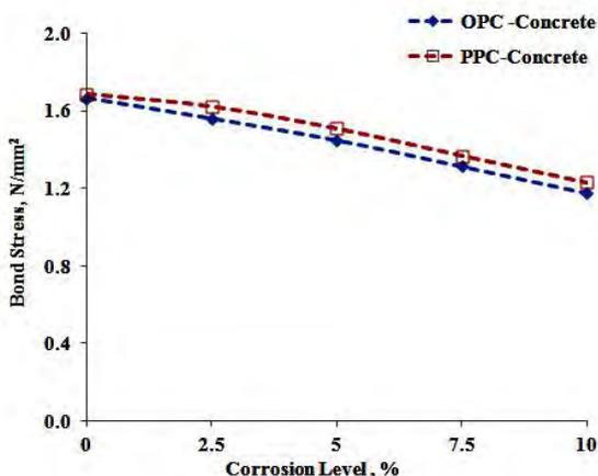
**Figure 16.** Effect of corrosion levels on bond stress of slip region at final strain values
