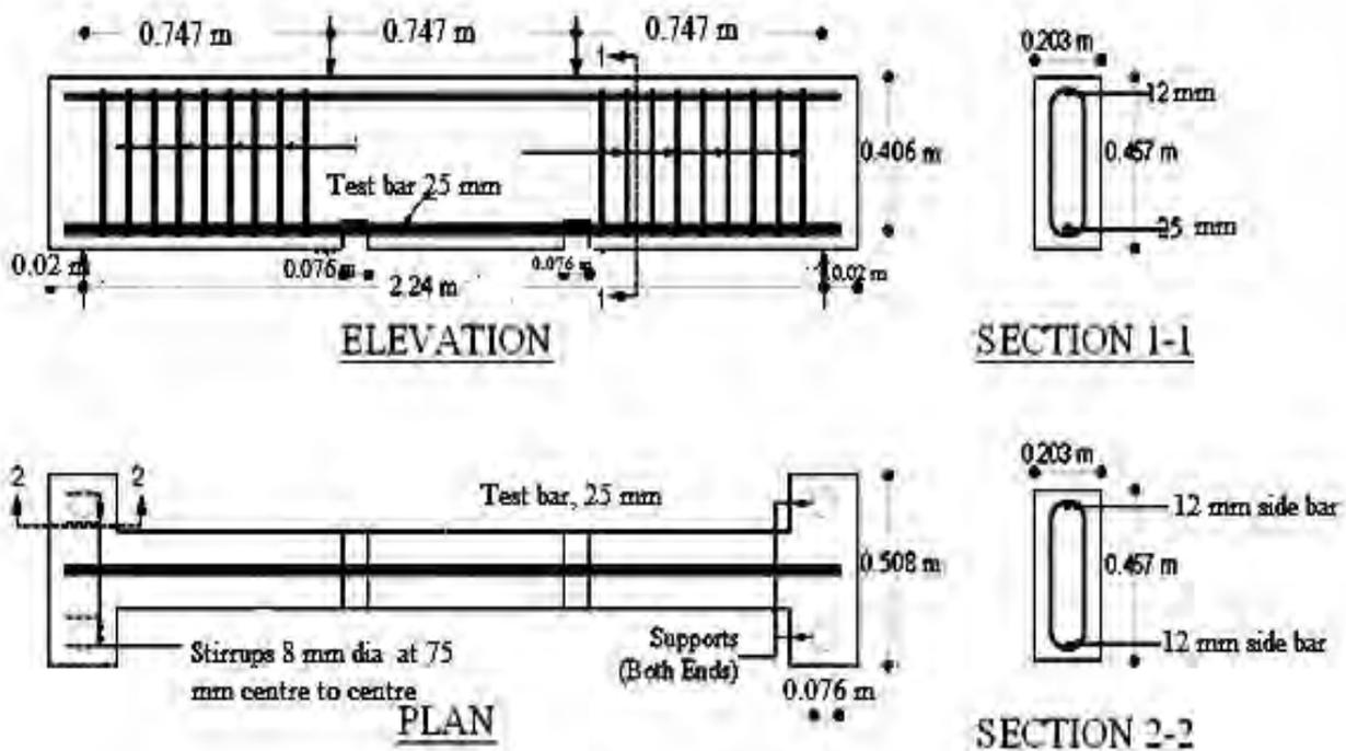
Figure 2. Reinforcement details of NBS beam specimen [11]
