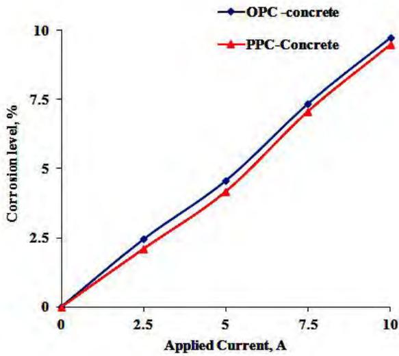
Figure 8. Variation of corrosion levels with Applied current
