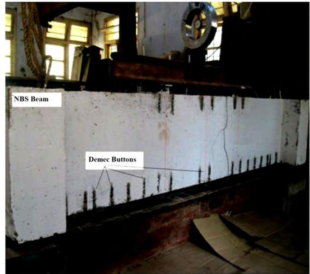
Figure 5(b). Demec buttons were at 100 mm c/c
