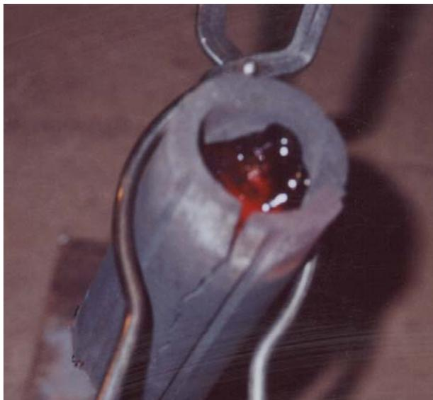
Figure 5. Molten basalt in carbon container
