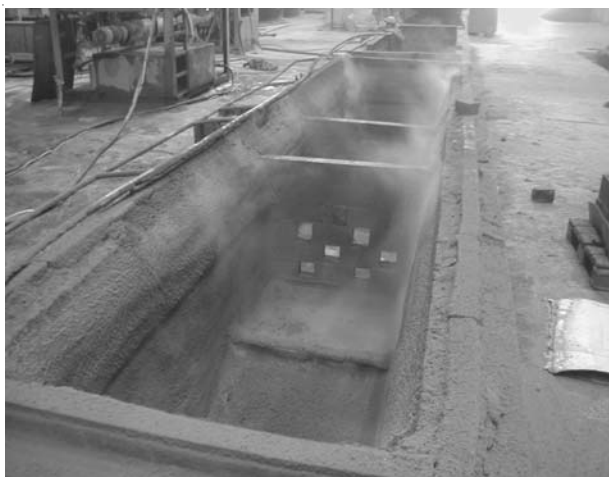
Figure 3. “B” tundish, equipped with flat impact pad & a pair of baffles & dams
