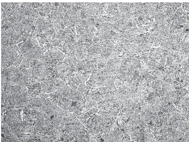
**Figure 2** Microstructure of the heat affected zone (100x)
