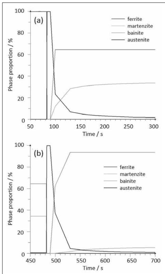
**Figure 10** Phases proportion development in node no. 25 190: a) after the 1<sup>st</sup> track, b) after the 2<sup>nd</sup> track
