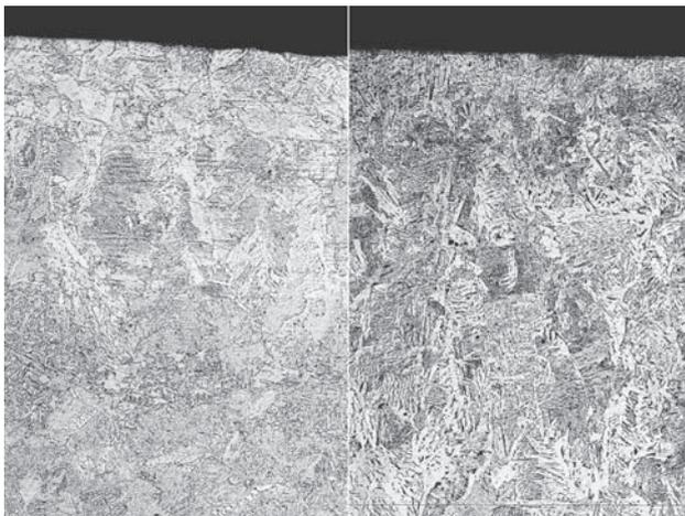
**Figure 1** Microstructure of the laser remelted zone: a) in the 1<sup>st</sup> track, b) in the 2<sup>nd</sup> track (100x)
