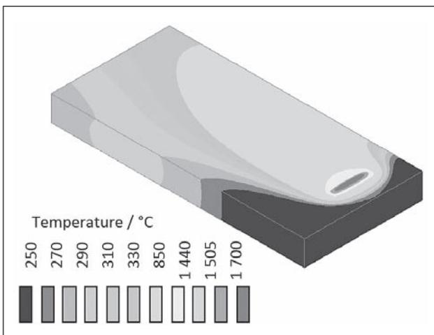
**Figure 7** Temperature distributions on the sample surface in the 490<sup>th</sup> sec.
