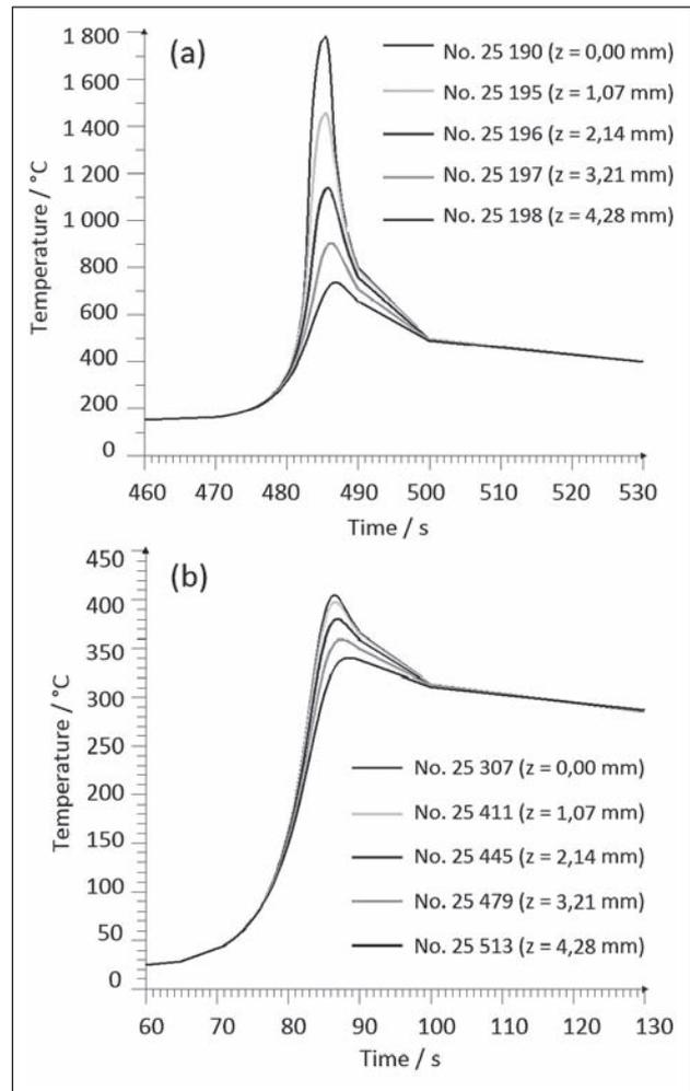
**Figure 8** Temperature histogram at five nodes of the vertical axis: a) an overlapped region, b) the 2<sup>nd</sup> track
