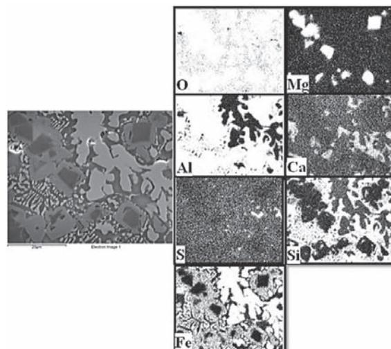
**Figure 6** Mapping of the alumina based deposit and entrapped steel
