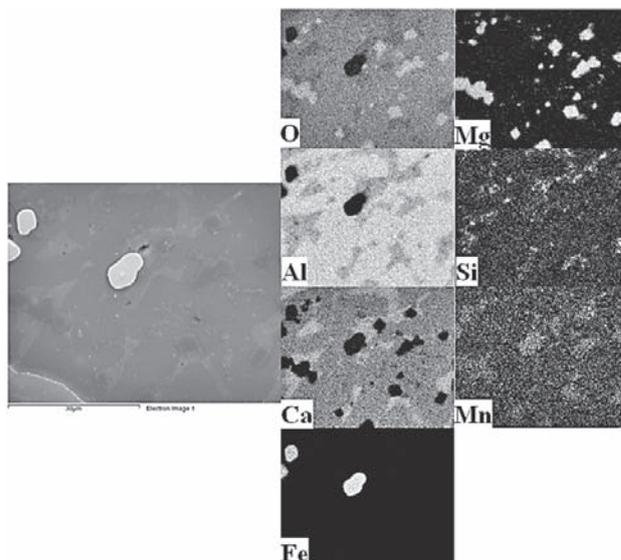
**Figure 5** Mapping of dense alumina based nozzle deposit
