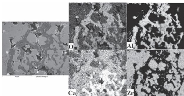
**Figure 3** Mapping of zirconia refractory with alumina inclusions
