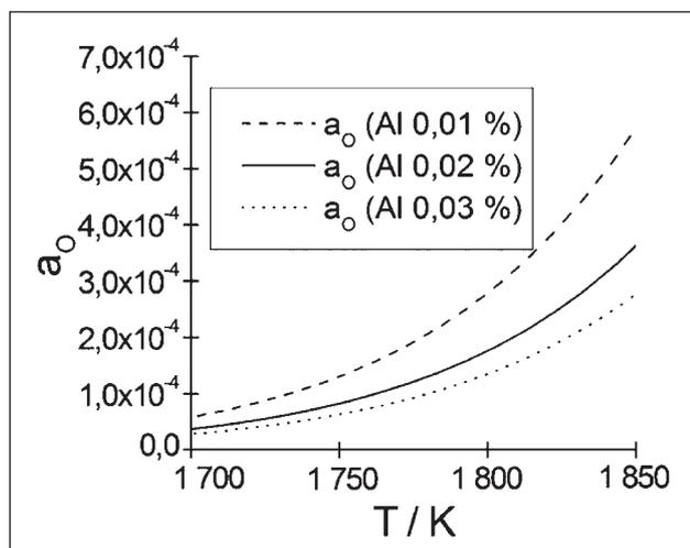
**Figure 4** Oxygen activity in steel melt for different temperatures
