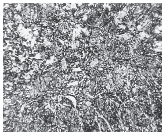
Figure 6 Filler material – sample 2, attack with Nital 2 / %; 100 ×
