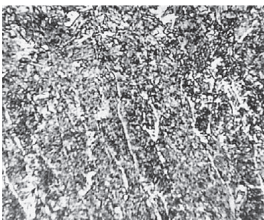
Figure 4 Heat affected zone, – sample 1, attack with Nital 2 / %; 100 ×
