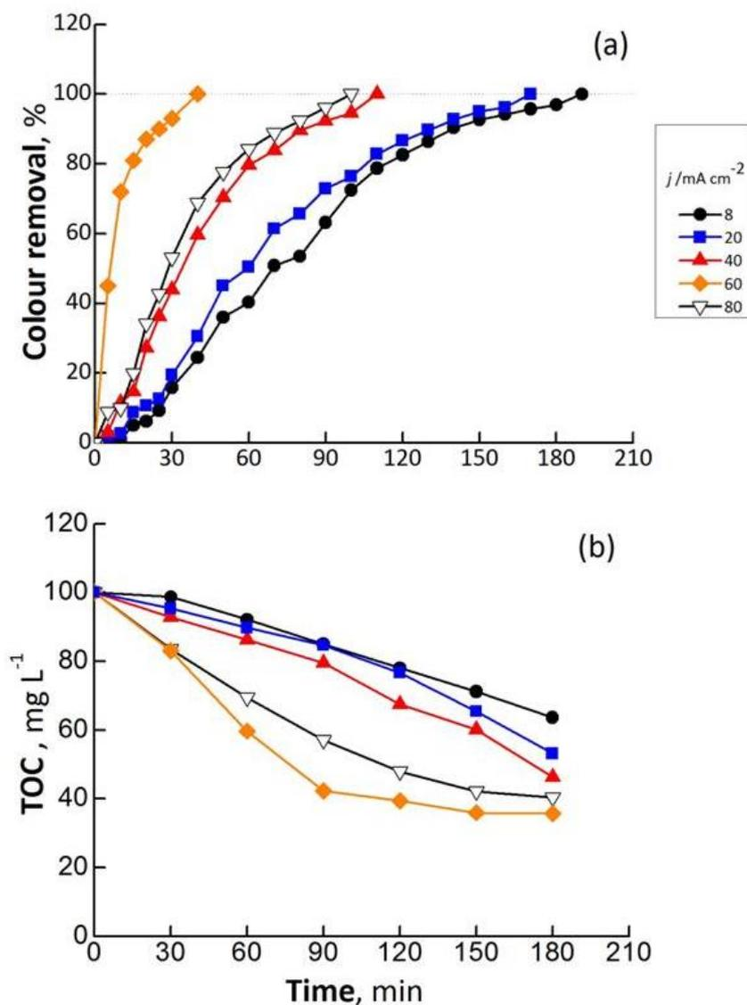
**Figure 2.** Effect of current density on (a) decolourization efficiency at 520 nm and (b) TOC removal with electrolysis time for the electro-Fenton treatment of solutions of 300 mg L<sup>-1</sup> AR1 in 0.05 M  $\text{Na}_2\text{SO}_4$  with 1.0 mM  $\text{Fe}^{2+}$  at pH 3.0 and 35 °C.
