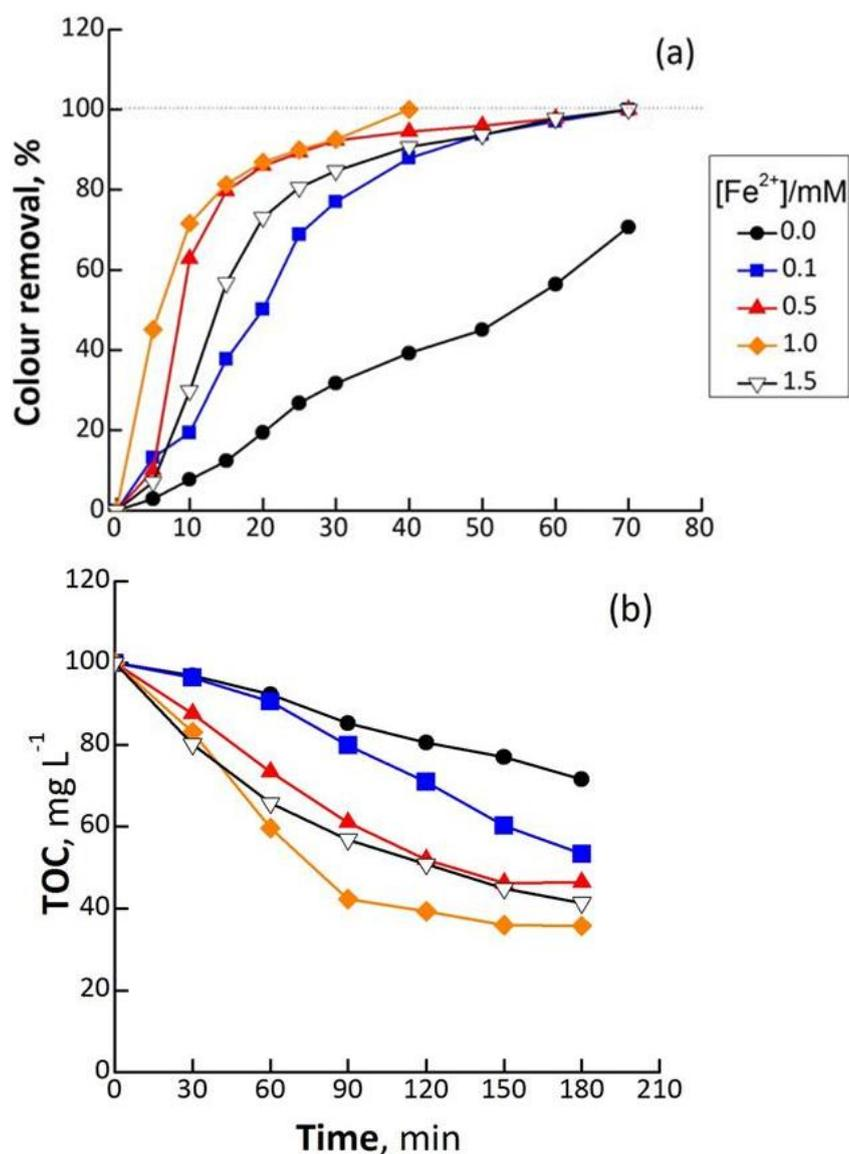
**Figure 1.** Effect of  $\text{Fe}^{2+}$  concentration on (a) decolourization efficiency at 520 nm and (b) TOC removal with electrolysis time for the electro-Fenton treatment of solutions of  $300 \text{ mg L}^{-1}$  AR1 in  $0.05 \text{ M Na}_2\text{SO}_4$  at pH 3.0,  $35 \text{ }^\circ\text{C}$  and  $60 \text{ mA cm}^{-2}$ .
