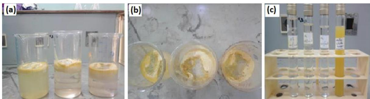
**Figure 2.** Foam formation: (a) face view, (b) top view. (c) Initial and final state of a 200 mg L<sup>-1</sup> DY solution treated by EC during 1 h: from right to left, initial solution, treated solution at 12, 8 and 4 V, respectively.
