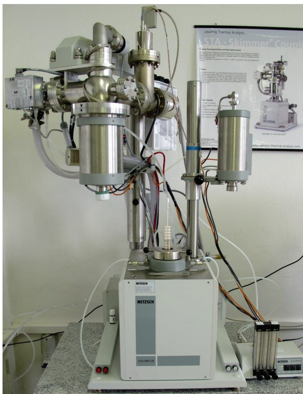
Figure 1 Netzsch STA 409CD – Simultaneous Thermal Analysis Apparatus
