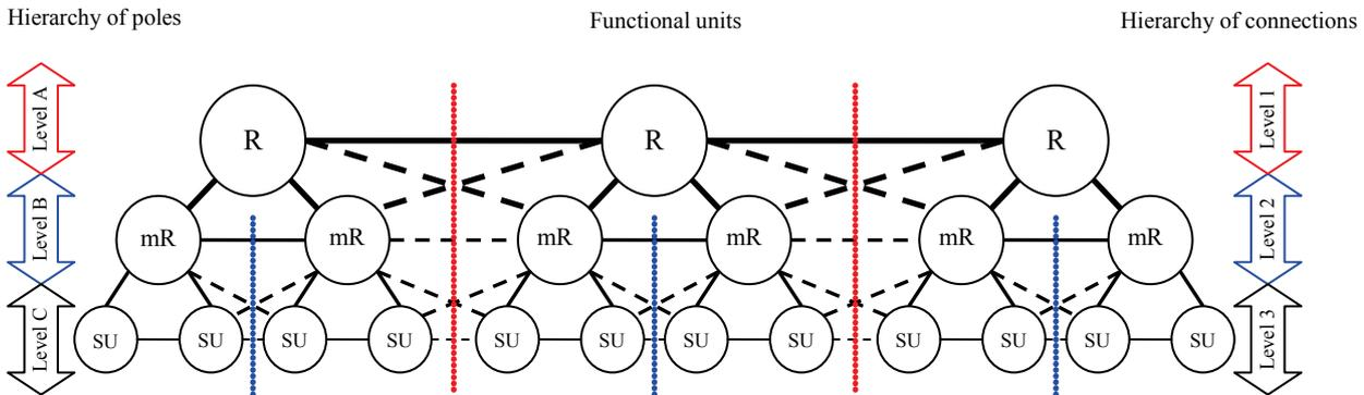
Figure 6 The structure of the road transport network according to Schönharting and Pischner (1983) [10]
