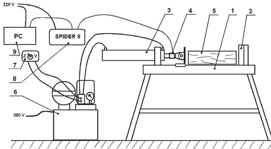
**Figure 2** Horizontal splitter with measuring chain (1 – frame of horizontal splitter, 2 –splitting wedge, 3 – straightforward hydraulic engine, 4 – strain gauges, 5 – splitting log, 6 – hydraulic unit, 7 – control panel, 8 – logger, 9 – personal computer (pc)
