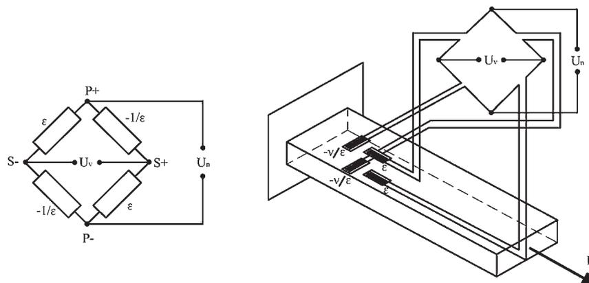
**Figure 3** Beam tensile stress - pressure – full bridge with complete compensation (Hoffmann, 1989)
