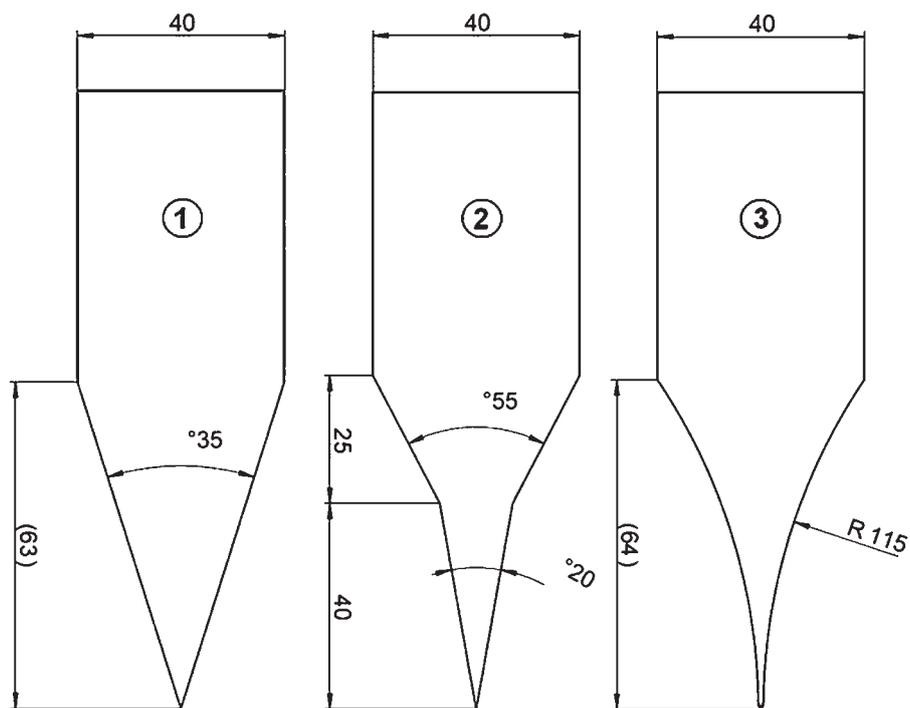
**Figure 4** Various shapes of splitting wedges (1 – simple splitting wedge, 2 – refracted splitting wedge, 3 – concave splitting wedge)
