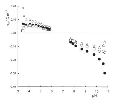
Figure 3. Effect of the initial pH value on the calculated values of the surface charge for two sets of experimental data taken from Figure 1. Acidic region: pH (initial) =  $3.4 (\diamond)$ ;  $3.33^* (\diamond)$ ;  $3.2 (\Box)$ . Basic region:  $10.8 (\Delta)$ ;  $10.9^* (O)$ ;  $11.0 (\bullet)$ . The measured initial pH values are denoted by asterisk.
