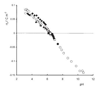
Figure 2. Surface charge density of hematite particles calculated by equation (16) from data presented in Figure 1, using the same symbols. The value of  $K_{\rm w} = 10^{-14}$  was used in calculations.
