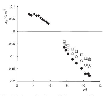
Figure 4. Effect of the chosen value of the equilibrium constant of the water dissociation constant  $K_w$  on the calculated values of the surface charge density for experiments presented in Figure 3. The following values were used:  $pK_w = 13.9 (\Box)$ ; 14.0 (O); 14.1 ( $\bullet$ ). In the acidic range ( $\bullet$ ), no difference was obtained for any assumed value of  $K_w$ . In the calculations, the measured initial pH values were used.
