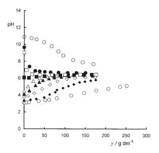
Figure 1. Mass titration of several experimental runs differing in the initial pH of the water to which hematite powder was added. Initial pH:  $3.1 (\bullet)$ ;  $3.3 (\bullet)$ ;  $3.7 (\diamond)$ ;  $4.1 (\blacktriangle)$ ;  $4.5 (\Delta)$ ;  $6.1 (\bullet)$ ;  $9.0 (\Box)$ ;  $9.6 (\bullet)$ ; 10.9 (O); Temperature 25.0 °C. Ionic strength:  $I = 0.001 \text{ mol dm}^{-3}$ .
