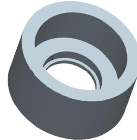
Figure 1. Three dimensional solid model of the bearing sleeve.
