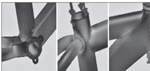
Figure 4 FEA results showing tensile and correlation to failure location
