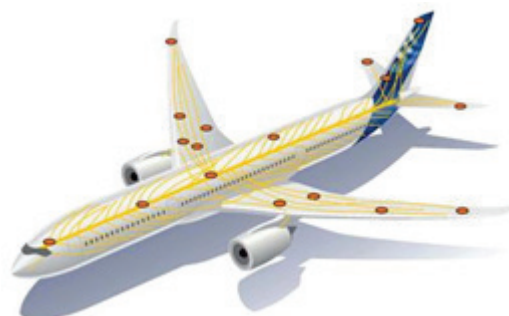
Figure 24 Structural health monitoring (SHM) systems can be arrayed in similar fashion to the human nervous system, with sensors concentrated in key areas where loads are highest [27]
