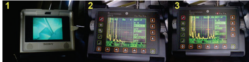
Figure 3 An example of Ultrasonic Testing (UT) on blade roots of a V2500 IAE aircraft engine (step 1: the UT probe is placed on the root of the blades to be inspected with the help of a special borescope tool (video probe), step 2: instrument settings are input, step 3: the probe is scanned over the blade root; an indication to the left of that range indicates a crack) [23]
