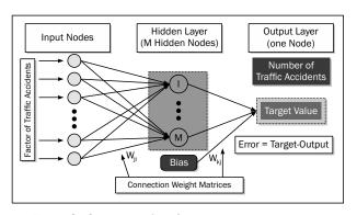
Figure 2 - Structure of artificial neural network model for traffic accidents
