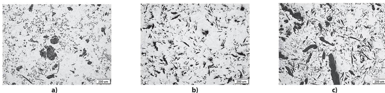
**Figure 2** Microstructure of: (a) CuSn10PTi2 composite containing 1,5 wt. % of graphite (20  $\mu\text{m}$ ), (b) CuSn10Ti0,4/graphite (45  $\mu\text{m}$ ) composite, (c) CuSn10Ti1,5/graphite (45  $\mu\text{m}$ ) composite
