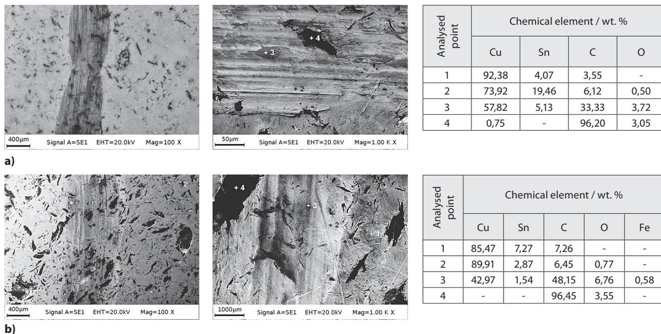
**Figure 3** SEM micrographs of the worn surfaces of: (a) CuSn10Ti0,4/graphite (45 µm), (b) CuSn10Ti1,5/graphite (45 µm) composite after interaction with a steel ball
