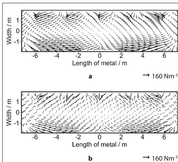
Figure 2 Horizontal electromagnetic force at 2/3 height of the metal pad /  $\text{Nm}^{-3}$  a) traditional cell b) novel cell
