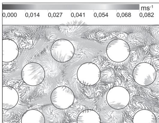
Figure 4 Sectional flow field in the middle of the metal pad in novel cell, t = 100 s
