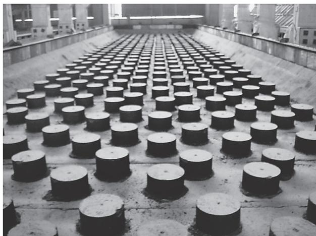
Figure 1 Novel cathode structure
