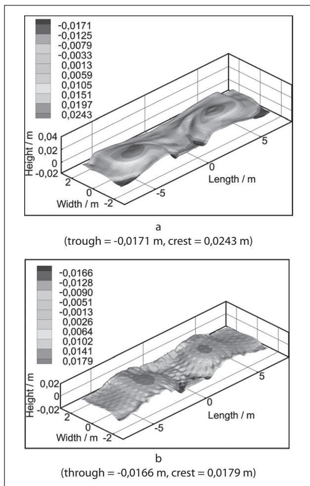
Figure 5 Metal - bath interface shape, t = 100 s
