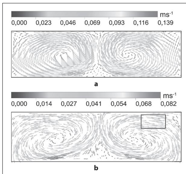
Figure 3 Flow field at 2/3 height of the metal pad,  $t = 100 \text{ s}$  a) traditional cell b) novel cell
