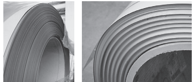
Figure 1 Coil winding errors
