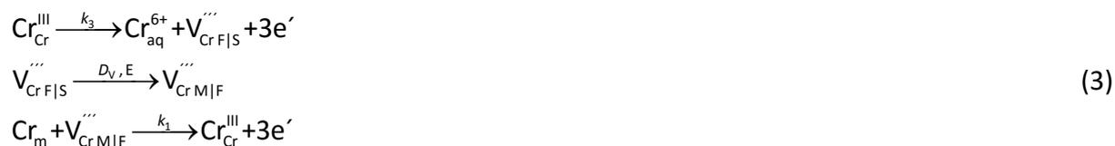
It can be in principle postulated that the dissolution of Mo through the film follows the same route as that of Cr, although at low potentials in the passivation region, the dissolution of Mo via the interstitial route probably cannot be neglected.
