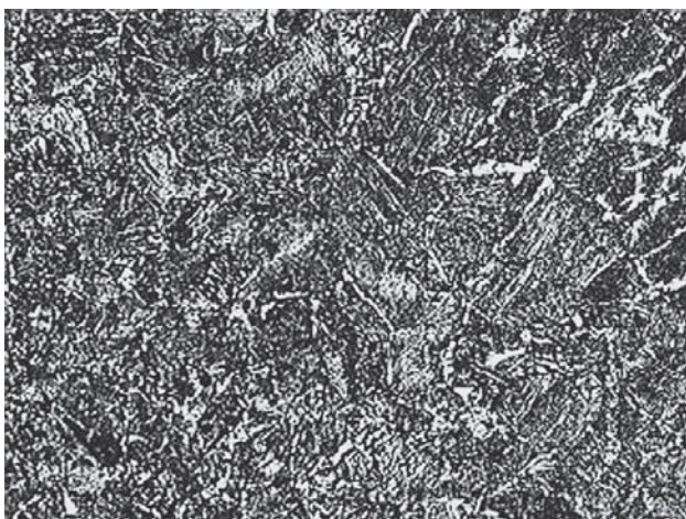
Figure 8 Weld near fusion line, Nital Etch, 100x, pearlitic-ferritic, Widmanstätten structure
