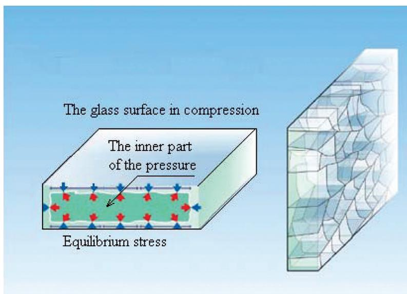
Figure 1 The glass surface in compression
