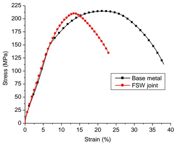
Figure 3. Strain-stress diagram for FSW joint and base metal.
