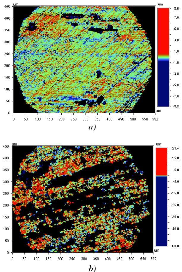
Figure 6. Corrosion surface: (a) WNZ, and (b) HAZ of friction stir weld joint of AA7039-O.
