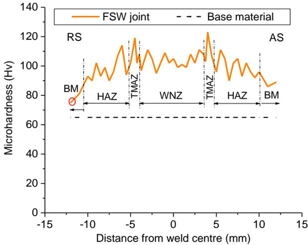
Figure 2. Microhardness variations across the FSW joint.
