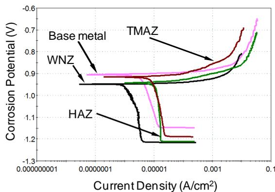
Figure 5. Potentiodynamic polarization curves for Tafel analysis in 3.5% NaCl solution.
