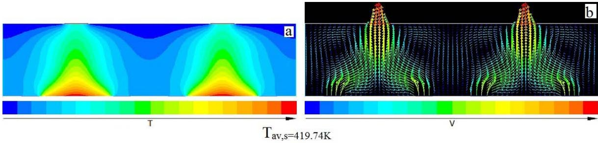
Fig.4 Obtained case for vents location on the lower plate: a. temperature contour, b. velocity vector.
