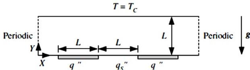
Fig.1 Schematic of 2D geometry and boundary conditions of two parallel plates without vents [11]
