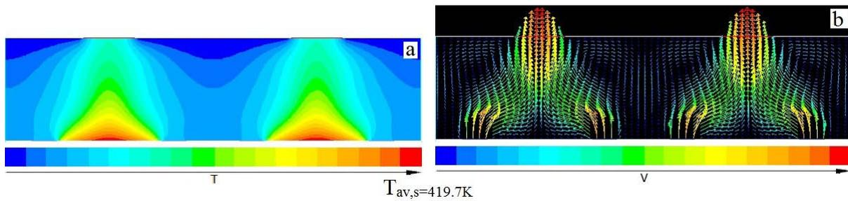
Fig.5 Obtained case for vents area on the upper and lower plates: a. temperature contour, b. velocity vector.
