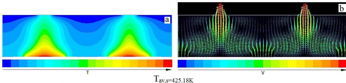
**Fig. 3** Obtained case for vents location on the upper plate: a. temperature contour, b. velocity vector.
