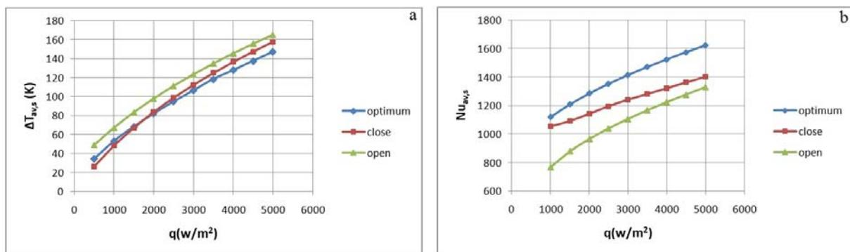
**Fig.7** Comparison among close, open and optimum case for different heat fluxes: a. temperature difference between cold plate and heat sources, b. mean Nusselt number at heat sources.
