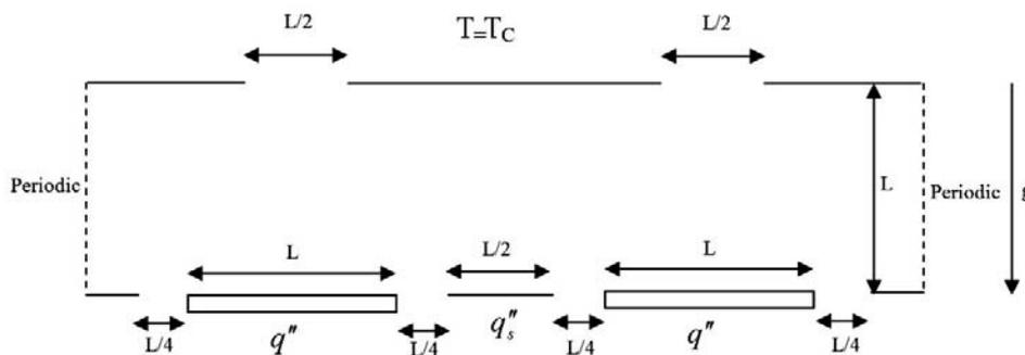
Fig. 6 Schematic of 2D geometry and boundary conditions of two parallel plates for the optimum case
