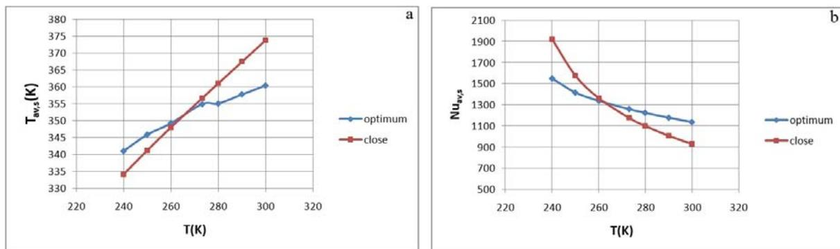
**Fig.8** Comparison between close and optimum case for different temperatures of cold plate with heat flux= $2000 \text{ w/m}^2$ : a. mean temperature on heat sources, b. mean Nusselt number on heat sources.
