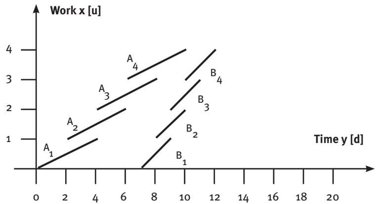
(a) LSM staggered with 2 crews (A:  $y_s = 0$  d,  $x_s = 0$  u,  $v_c = 1$  u/crew, lag time = -2 d (lead), slope =  $1/4$  u/d, time buffer = 0 d; B:  $y_s = 7$  d,  $x_s = 0$  u,  $v_c = 1$  u/crew, lag time = -1 d (lead), slope =  $1/2$  u/d).
