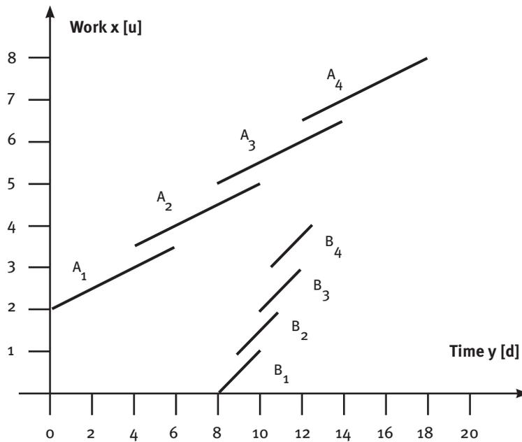
(d) LSM staggered with 2 crews (A:  $y_s = 0$  d,  $x_s = 2$  u,  $v_c = 1.5$  u/crew, lag time = -2 d (lead), slope =  $1/4$  u/d, time buffer = 0 d; B:  $y_s = 8$  d,  $x_s = 0$  u,  $v_c = 1$  u/crew, lag time = -1 d (lead), slope =  $1/2$  u/d).
