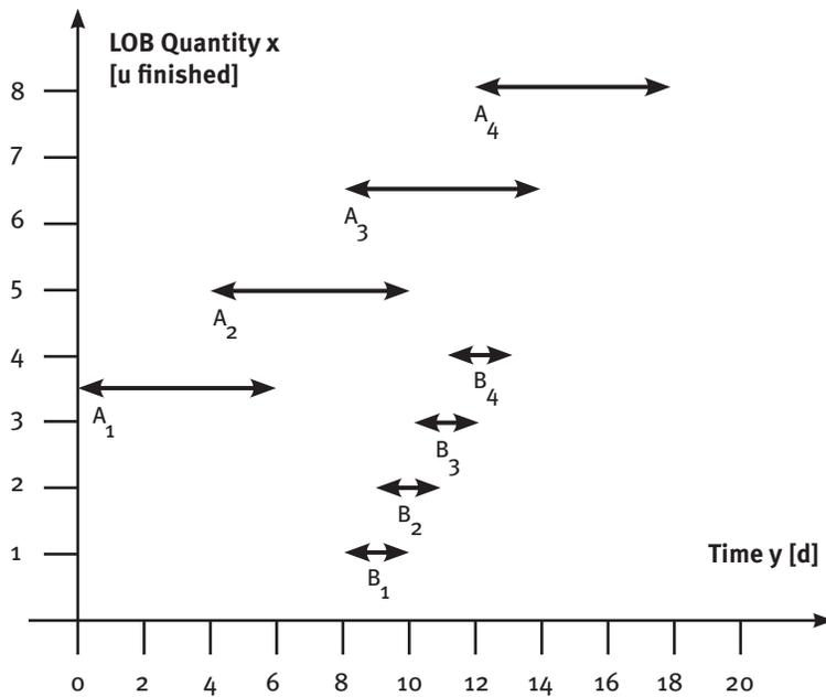
(d) LOB staggered with 2 crews (A:  $y_s = 0$  d,  $x_s = 2$  u,  $v_c = 1.5$  u/crew, lag time = -2 d (lead), task duration = 4 d, delivery rate =  $3/8$  u/d, time buffer = 0 d; B:  $y_s = 8$  d,  $x_s = 0$  u,  $v_c = 1$  u/crew, lag time = -1 d (lead), task duration = 2 d, delivery rate = 1 u/d).
