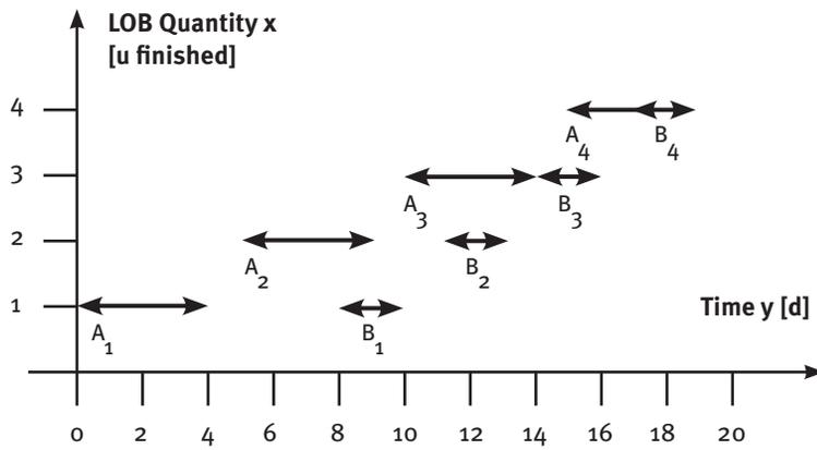
(c) LOB interruptible with 1 crew (A:  $y_s = 0$  d,  $x_s = 0$  u,  $v_c = 1$  u/crew, lag time = 1 d, task duration = 4 d, delivery rate =  $1/5$  u/d, time buffer = 0 d; B:  $y_s = 8$  d,  $x_s = 0$  u,  $v_c = 1$  u/crew, lag time = 1 d, task duration = 2 d, delivery rate =  $1/3$  u/d).
