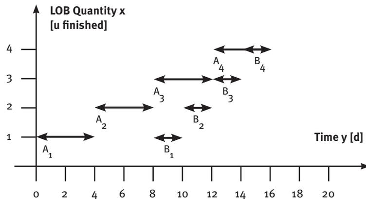
(b) LOB continuous with 1 crew (A:  $y_s = 0$  d,  $x_s = 0$  u,  $v_c = 1$  u/crew, task duration = 4 d, delivery rate =  $1/4$  u/d, time buffer = 0 d; B:  $y_s = 8$  d,  $x_s = 0$  u,  $v_c = 1$  u/crew, task duration = 2 d, delivery rate =  $1/2$  u/d).
