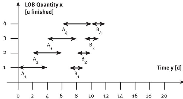
(a) LOB staggered with 2 crews (A:  $y_s = 0$  d,  $x_s = 0$  u,  $v_c = 1$  u/crew, lag time = -2 d (lead), task duration = 4 d, delivery rate =  $1/2$  u/d, time buffer = 0 d; B:  $y_s = 7$  d,  $x_s = 0$  u,  $v_c = 1$  u/crew, lag time = -1 d (lead), task duration = 2 d, delivery rate = 1 u/d).
