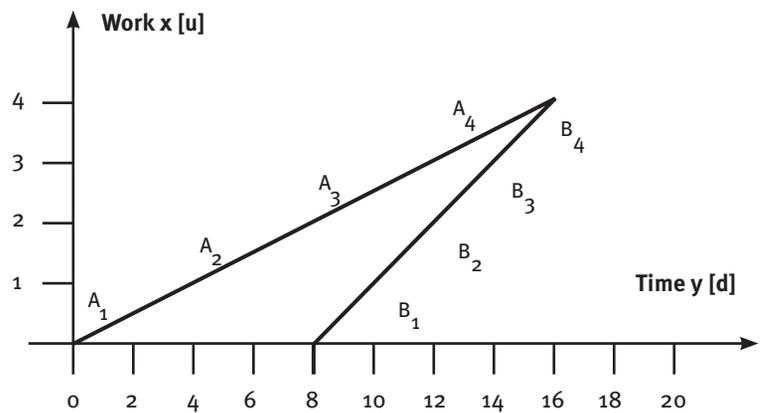
(b) LSM continuous with 1 crew (A:  $y_s = 0$  d,  $x_s = 0$  u,  $v_c = 1$  u/crew, slope =  $1/4$  u/d, time buffer = 0 d; B:  $y_s = 8$  d,  $x_s = 0$  u,  $v_c = 1$  u/crew, slope =  $1/2$  u/d).
