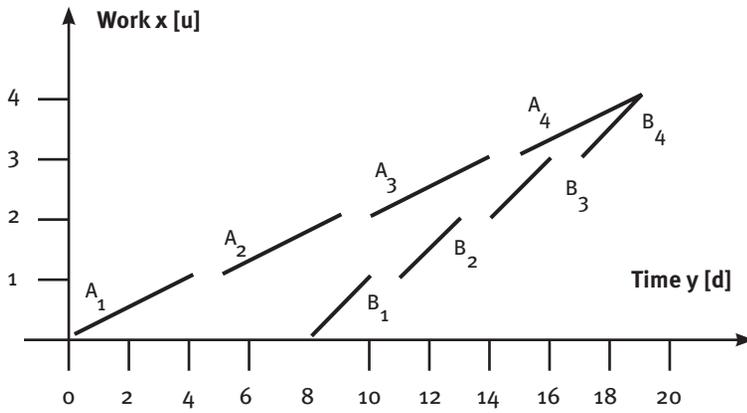
(c) LSM interruptible with 1 crew (A:  $y_s = 0$  d,  $x_s = 0$  u,  $v_c = 1$  u/crew, lag time = 1 d, slope =  $1/4$  u/d, time buffer = 0 d; B:  $y_s = 8$  d,  $x_s = 0$  u,  $v_c = 1$  u/crew, lag time = 1 d, slope =  $1/2$  u/d).
