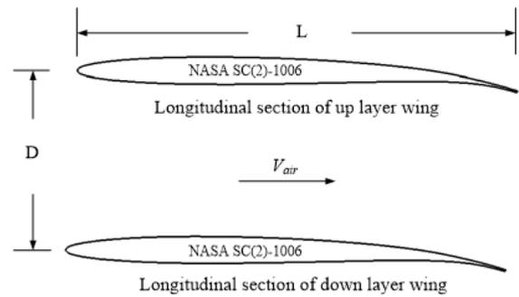
Figure 2. Longitudinal section of axial ring wing configuration.
