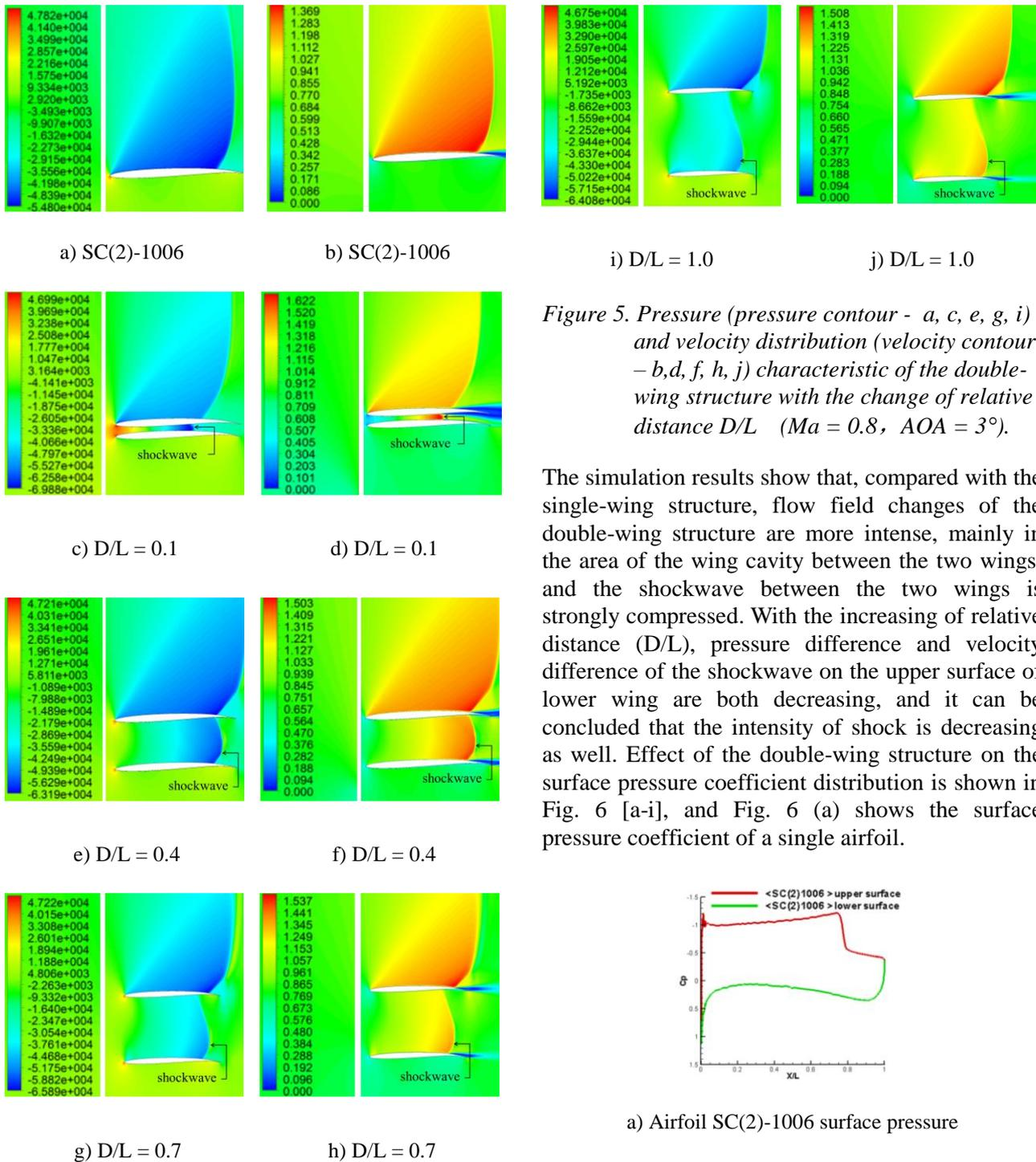
Figure 5. Pressure (pressure contour - a, c, e, g, i) and velocity distribution (velocity contour - b, d, f, h, j) characteristic of the double-wing structure with the change of relative distance  $D/L$  ( $Ma = 0.8$ ,  $AOA = 3^\circ$ ).
