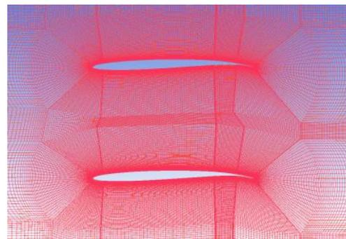
Figure 4. Partial double O Grid (D/L = 0.7).
