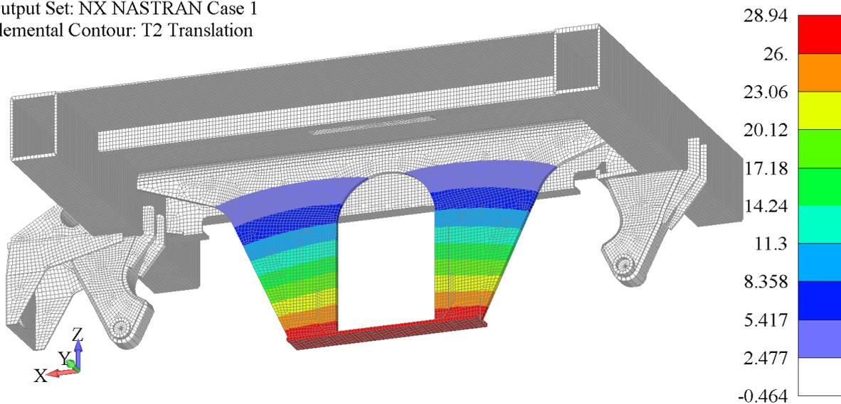
**Fig. 10** Lateral displacement field –  $U_y$  – model with new optimized shape of axle guard
