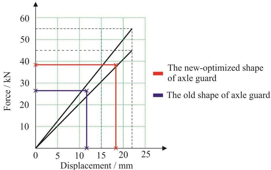
Fig. 11 Rigidity of axle guards at von Mises equivalent stress of 345 MPa
