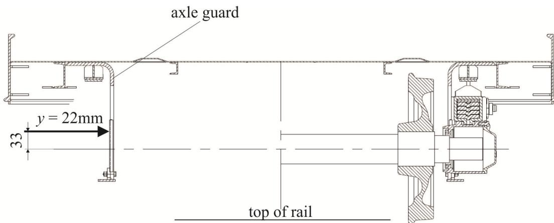
Fig. 12 Scheme of model loading; maximum lateral displacement  $y = 22$  mm
