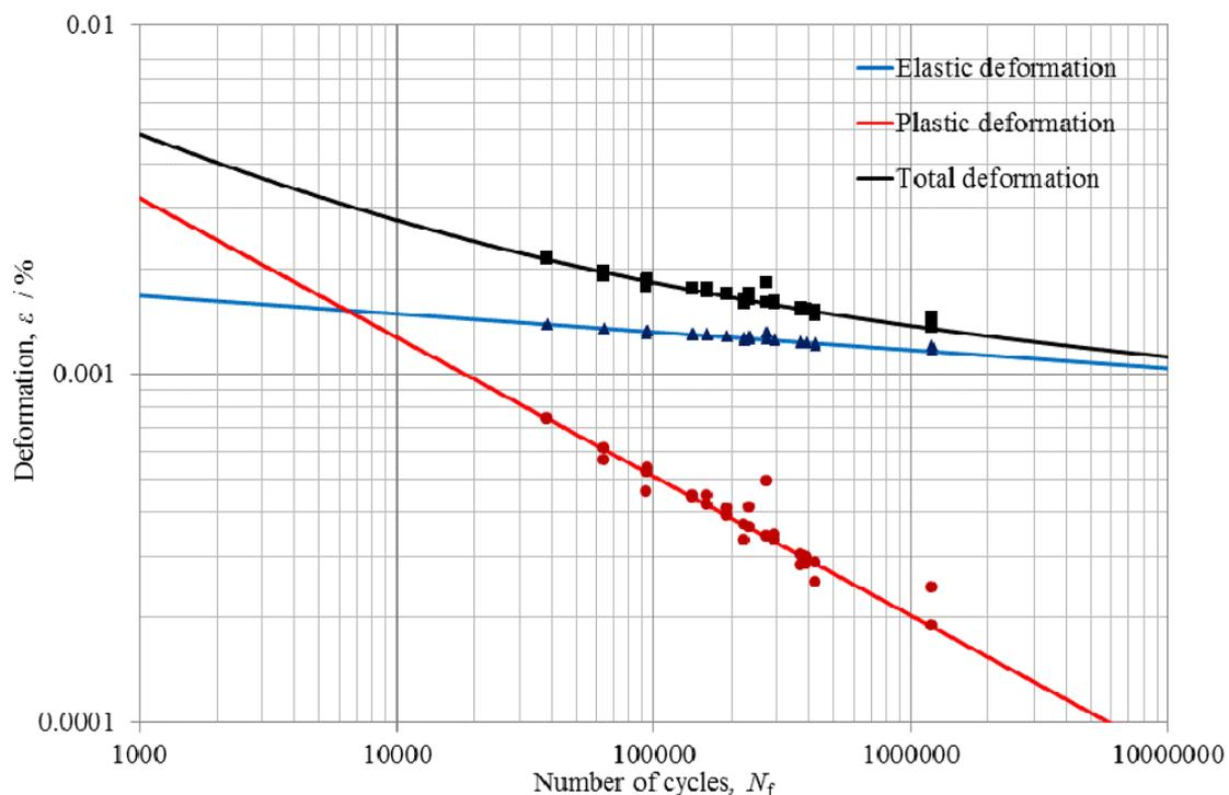
**Fig. 2** Strain–life curve resulting from uniaxial tension–compression fatigue tests of S355J2+N material
