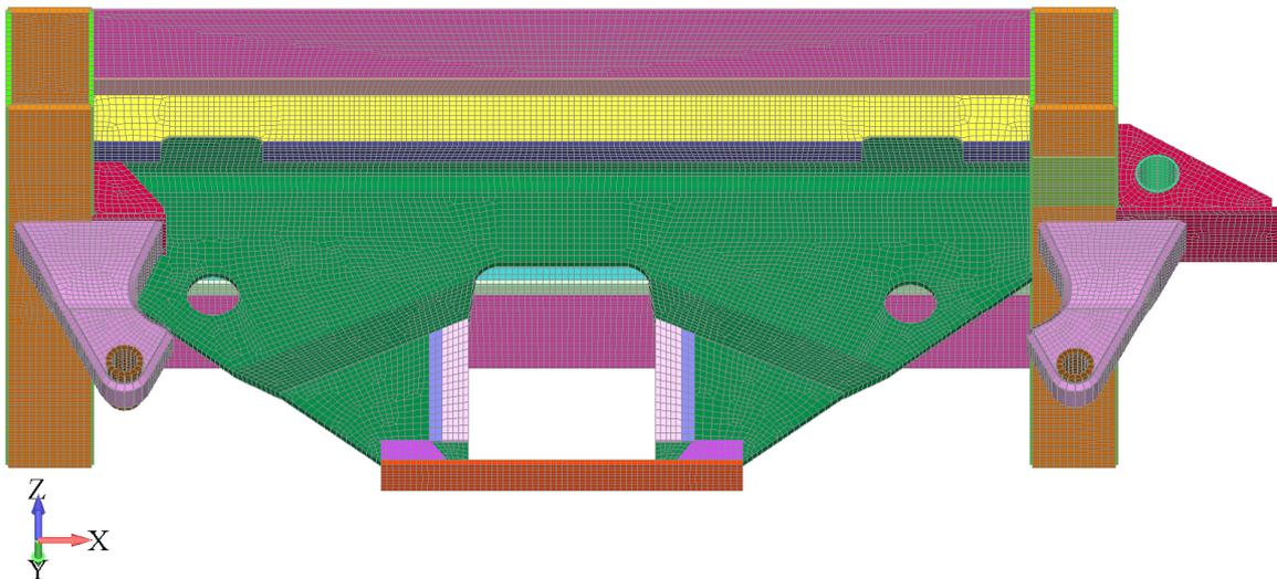
**Fig. 5** 3D model of running gear of Hccrrs 2x2 axle car-carrying wagon with old shape of axle guard – finite element mesh
