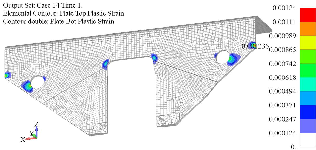
**Fig. 15** Plastic strain field –old shape of axle guard
