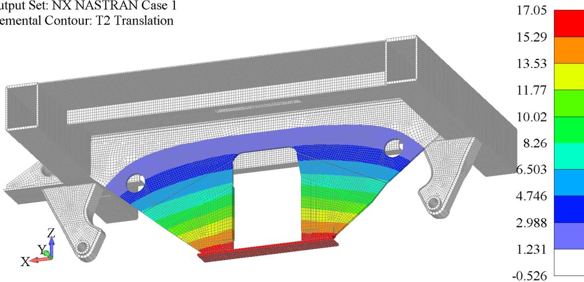
**Fig. 9** Lateral displacement field –  $U_y$  – model with old shape of axle guard
