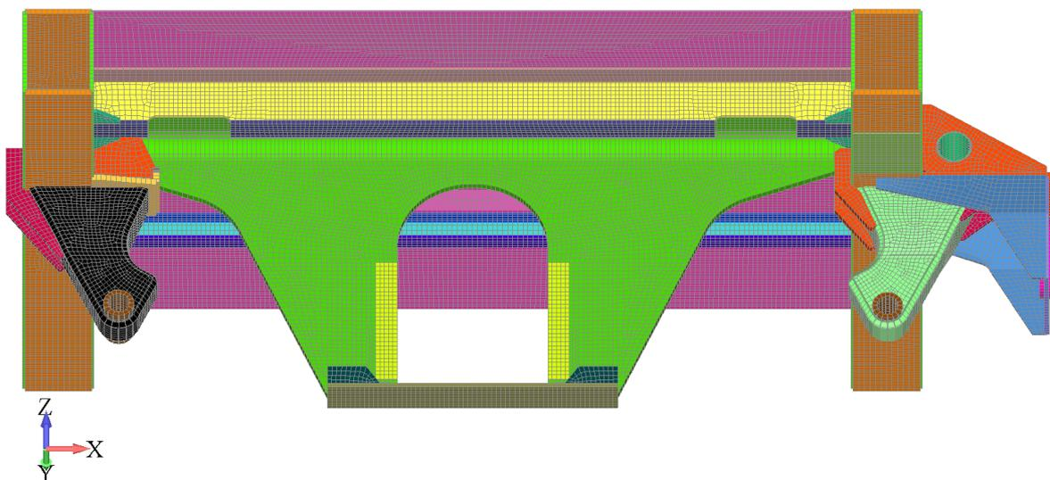
**Fig. 6** 3D model of running gear of Hccrrs 2x2 axle car-carrying wagon with new optimized shape of axle guard – finite element mesh
