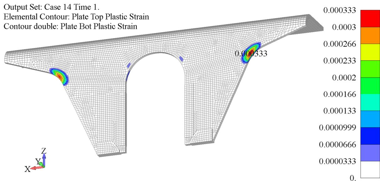
**Fig. 16** Plastic strain field –new optimized shape of axle guard
