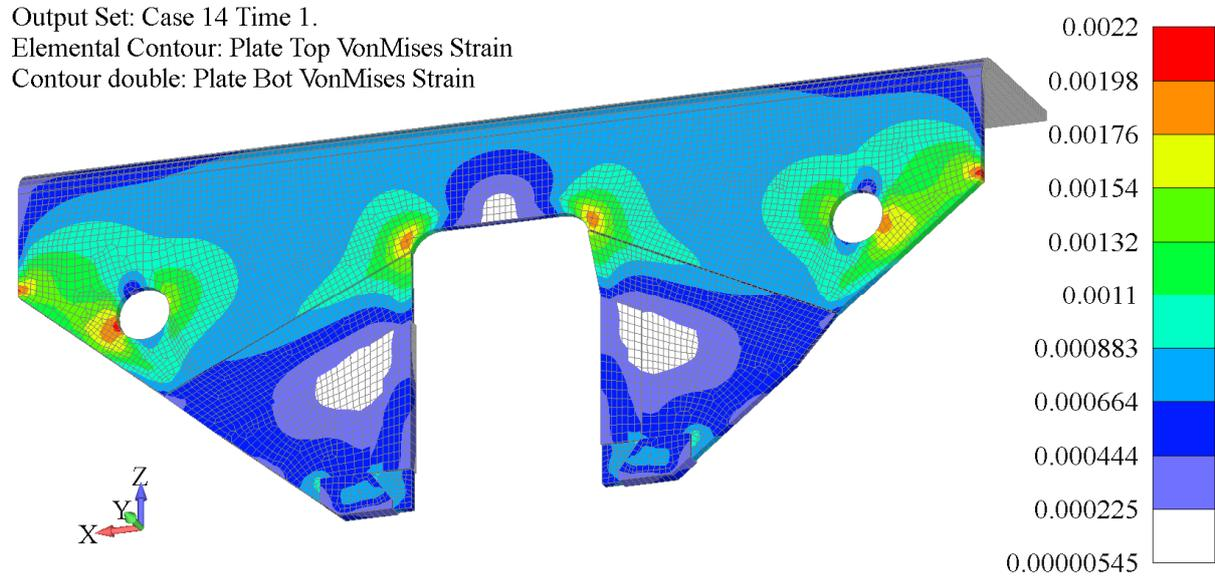
Fig. 13 Total strain field –old shape of axle guard
