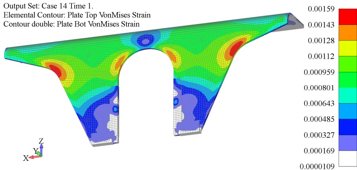
Fig. 14 Total strain field –new optimized shape of axle guard
