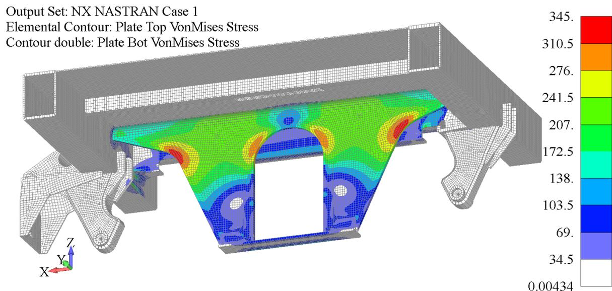
**Fig. 8** Von Mises equivalent stress field - model with new optimized shape of axle guard
