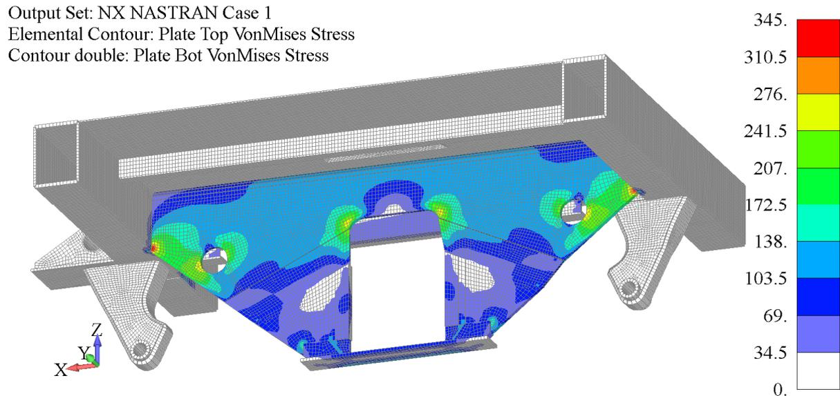
**Fig. 7** Von Mises equivalent stress field - model with old shape of axle guard
