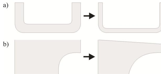
**Fig. 1** Types of optimization: a) parametric optimization, b) shape optimization
