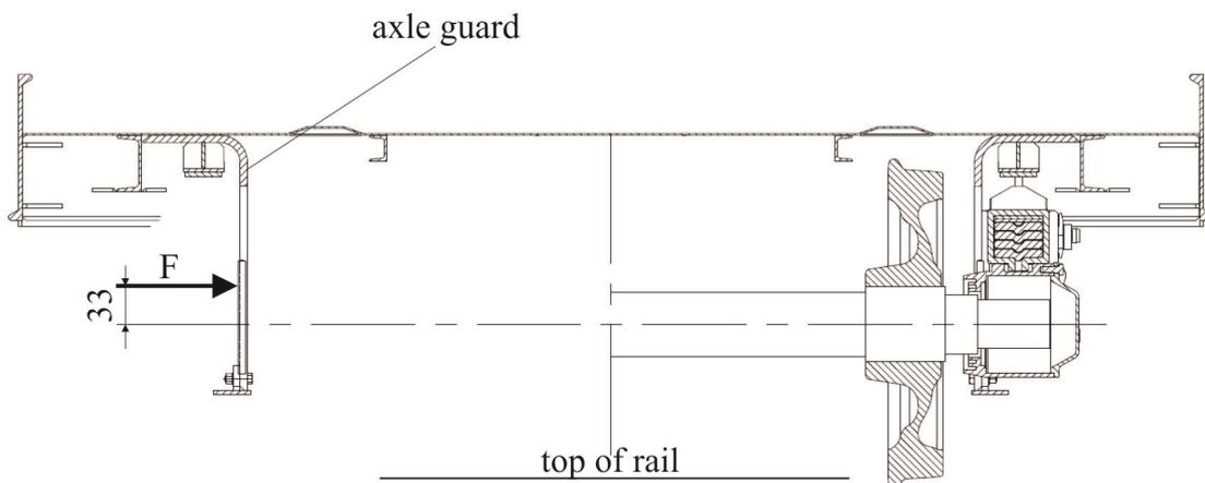
Fig. 4 Scheme of model loading; maximum lateral force for maximum stress of 345 MPa
