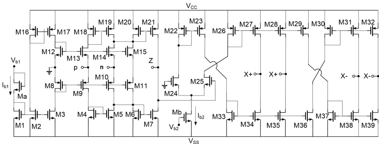
Fig. 2. The CDTA in this work
