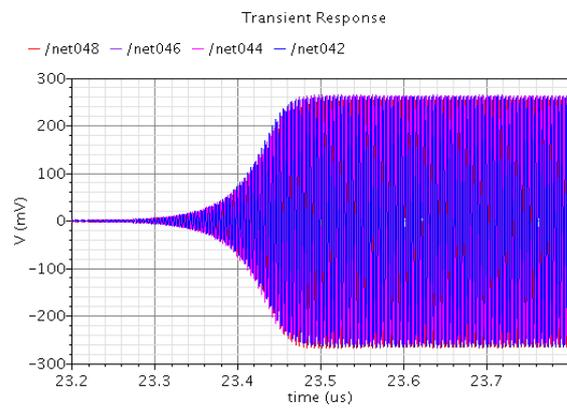
(a)  $v_{o1}$ ,  $v_{o2}$ ,  $v_{o3}$  and  $v_{o4}$  during initial state
