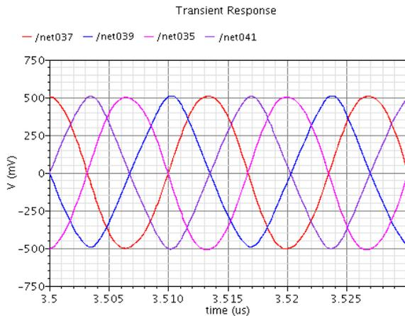
(b)  $v_{o1}$ ,  $v_{o2}$ ,  $v_{o3}$  and  $v_{o4}$  during initial state
