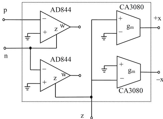
Fig. 9. Possible implementation of CDTA using commercially available ICs
