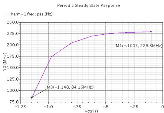
(b) The output frequency versus the bias voltage of the second TOQO
