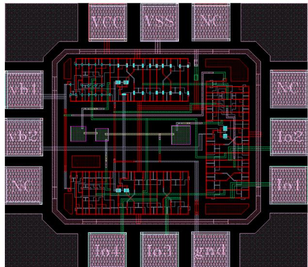
(b) The Layout of second TOQO in Fig.4 ( $1.2 \times 1.2\text{mm}^2$ )
