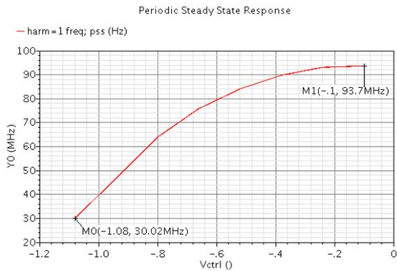
(a) The output frequency versus the bias voltage of the first TOQO
