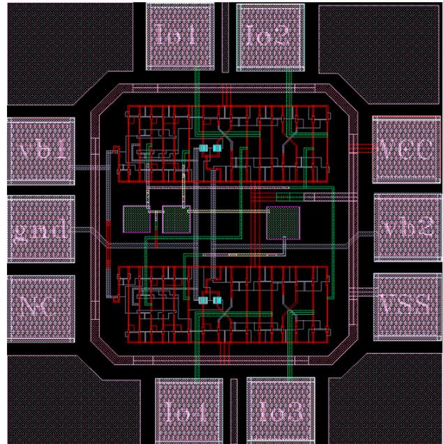
(a) The layout of first TOQO in Fig.3 ( $1.0 \times 1.0\text{mm}^2$ )
