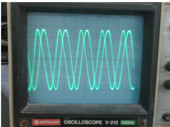
Fig. 10. Experimental evidence of the quadrature outputs
