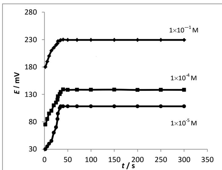
**Figure 5.** Response time of electrode*Lifetime*
