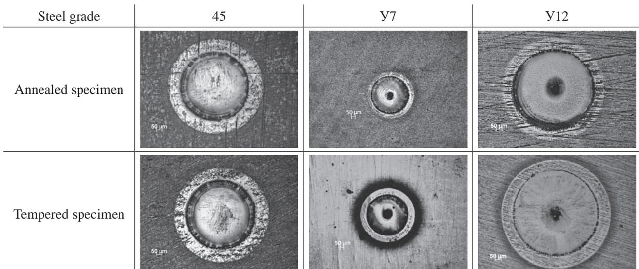
**Figure 2** Structure of laser-treated specimens with power density 31,2 kW/cm, plane section (001)
