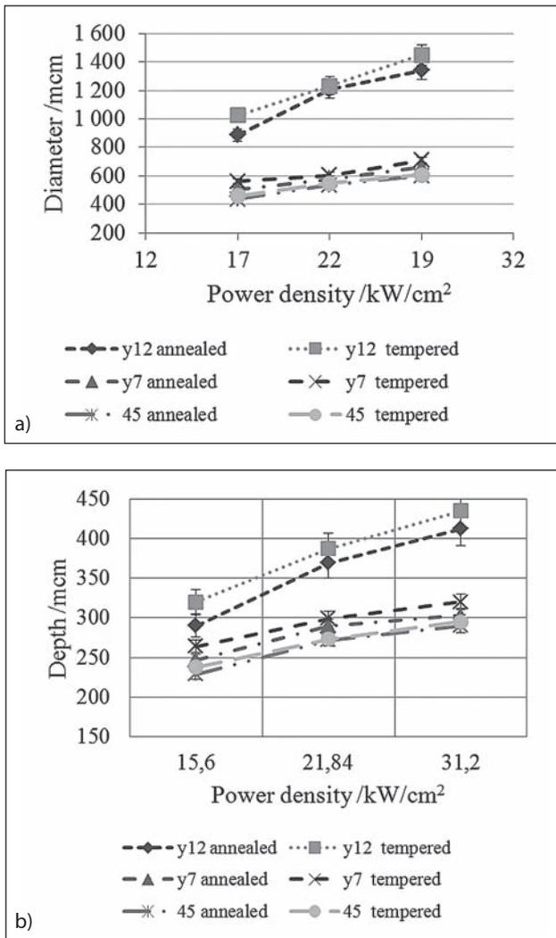
**Figure 3** Dependence of the laser effect zone diameter and depth on radiation power density and steel preliminary treatment
