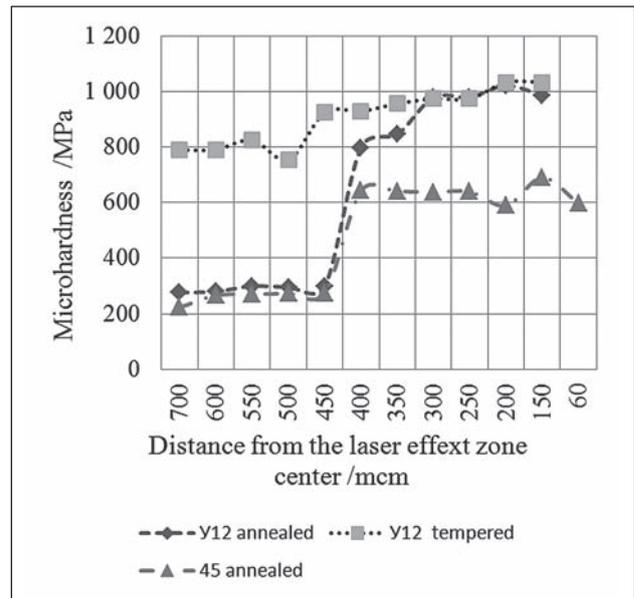
**Figure 4** Microhardness changing in the zone subject to laser treatment with power density 21,8 kW/cm²
