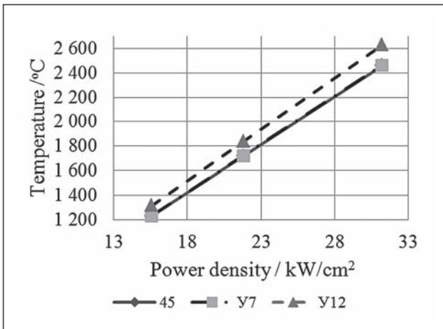
**Figure 1** Temperature achieved within the laser effect zone depending on radiation power density
