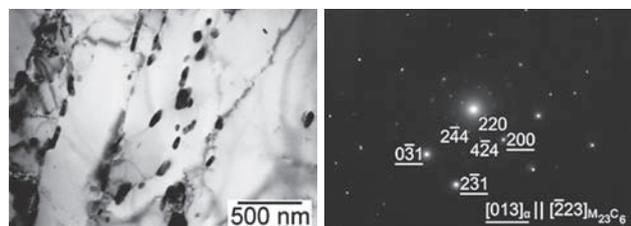
**Figure 5** Morphology of  $M_{23}C_6$  carbides observed in the CGHAZ area of the joint subjected to PWHT: a) bright visual field; b) SAED diffraction pattern of  $M_{23}C_6$  carbides:  $[013]_{\alpha} || [223]_{M_{23}C_6}$
