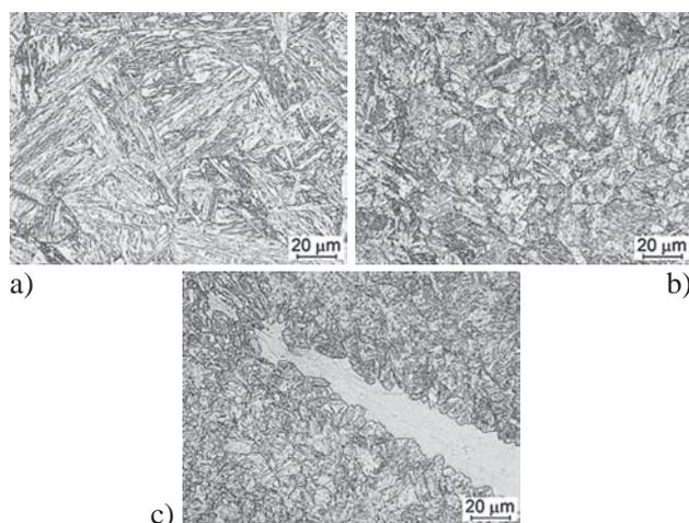
**Figure 2** Microstructure of the joint not subjected to PWHT, i.e. welded using the TBT: a) PB2 steel parent metal: tempered martensite; b) CGHAZ: tempered martensite; c) weld: tempered martensite + delta ferrite; etchant:  $\text{FeCl}_3$ , mag. 500x
