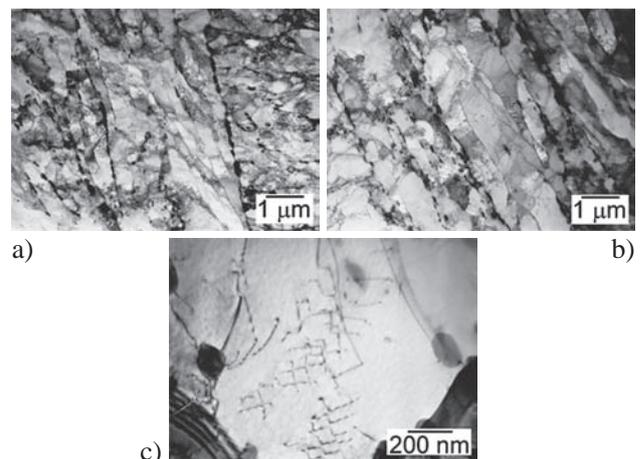
**Figure 4** Microstructures observed on the thin films (TEM) in the CGHAZ area of the joint welded using the TBT: a) general morphology of tempered martensite; b) morphology of ferrite subgrains; c) dislocation density in subgrains
