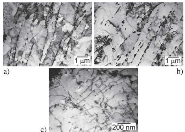
**Figure 3** Microstructures observed on the thin films (TEM) in the CGHAZ area of the joint subjected to PWHT: a) general morphology of tempered martensite; b) morphology of ferrite subgrains; c) dislocation density in subgrains
