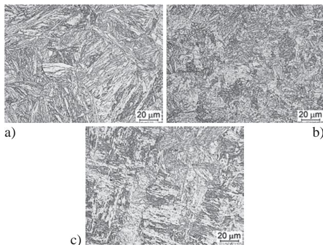
**Figure 1** Microstructure of the joint subjected to PWHT: a) PB2 steel parent metal: tempered martensite; b) coarse-grained HAZ (CGHAZ): tempered martensite; c) weld: tempered martensite; etchant:  $\text{FeCl}_3$ , mag. 500x
