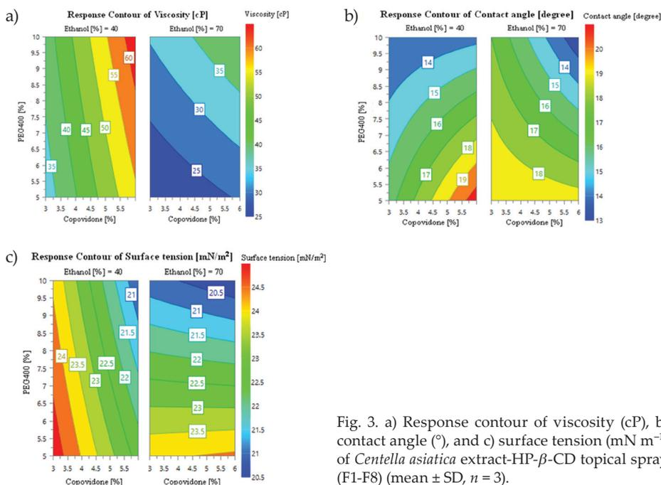
Fig. 3. a) Response contour of viscosity (cP), b) contact angle ( $^{\circ}$ ), and c) surface tension ( $\text{mN m}^{-1}$ ) of *Centella asiatica* extract-HP- $\beta$ -CD topical spray (F1-F8) (mean  $\pm$  SD,  $n = 3$ ).
