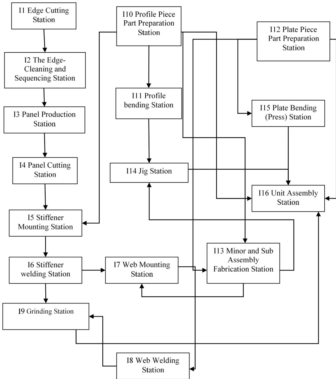
**Figure 2** Workflow chart of the work stations in the ship production process [18]
