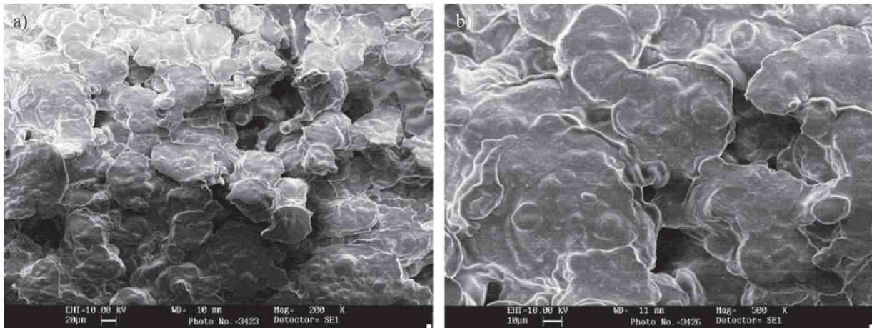
**Fig. 2.** Scanning electron photomicrograph showing calcium alginate and starch beads coated with chitosan layer at magnification of: a) 200× and b) 500×
