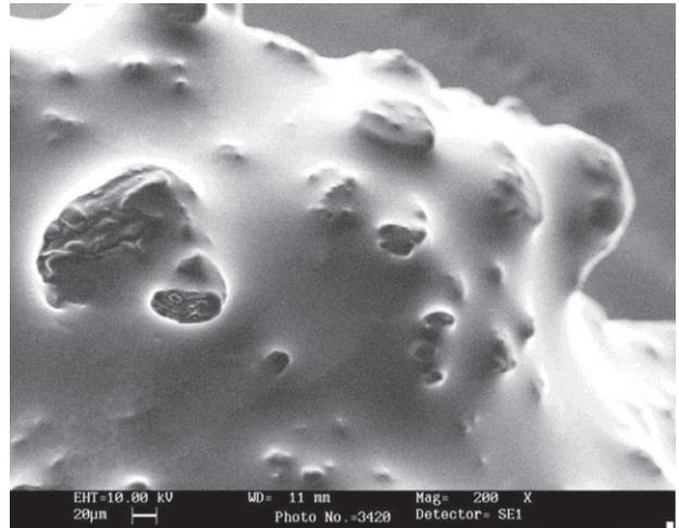
**Fig. 1.** Scanning electron photomicrograph showing calcium alginate and starch beads at magnification of 200 $\times$
