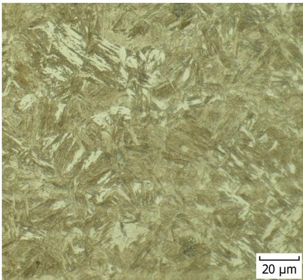
Figure 1. Microstructure of Hardox 500 in “as delivered” state.
