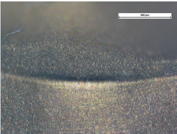
Figure 3. Surface morphology of cutting tool edge geometry before the start of milling (50x).
