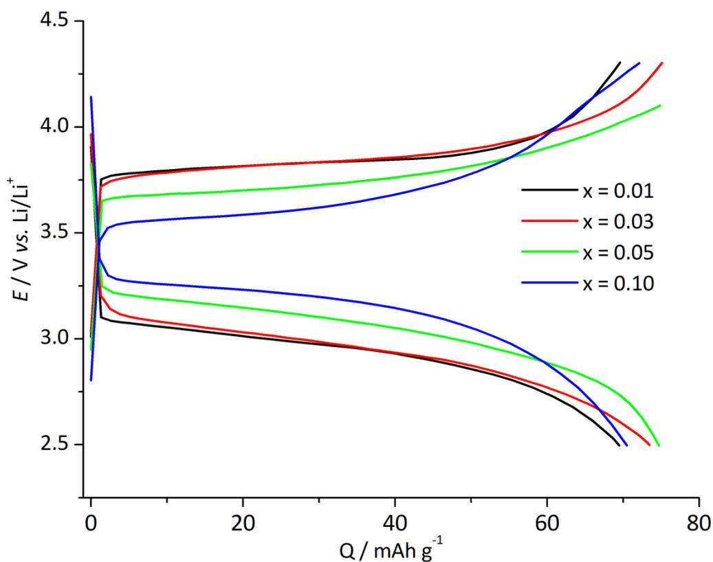
**Figure 3.** Charge-discharge curves for  $\text{LiFe}_{1-x}\text{V}_x\text{PO}_4$  ( $x = 0.01, 0.03, 0.05, 0.1$ ):
