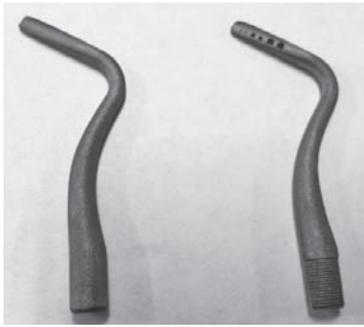
Figure 1 Beaks of elevators sintered by DMLS
