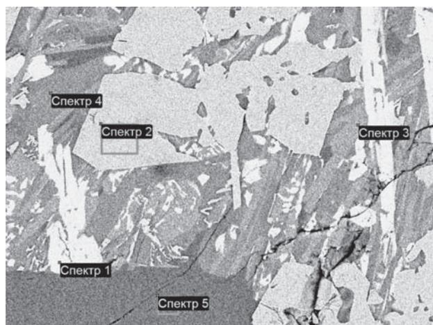
Figure 6 Microstructure of CAMS alloy through electron microscope JEOL-JSM7001F with an increase of 400 mkm
