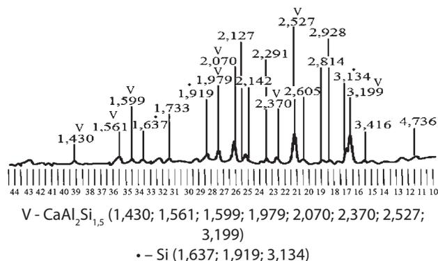
Figure 1 XRD pattern of a metal No. 1
