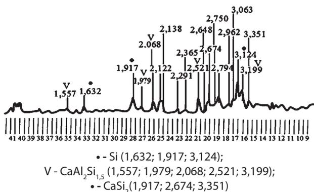
**Figure 3** XRD pattern of a metal No. 3
