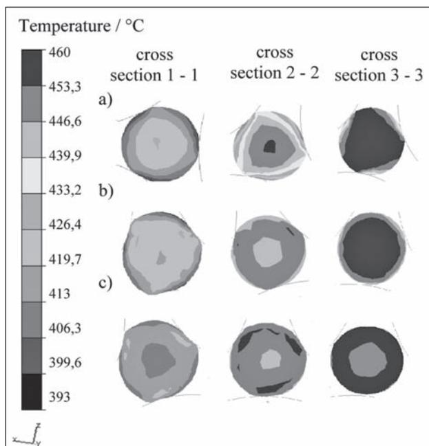
**Figure 5** Temperature distributions in cross-sections of the rolled bar during the rolling of ingot with diameter of  $\phi$  30 mm to the bar with diameter of  $\phi$  24 mm with temperature of 400 °C and rotational speed of the rolls of: a)  $n_w = 25$  rev/min, b)  $n_w = 75$  rev/min, c)  $n_w = 100$  rev/min
