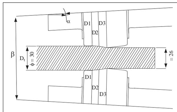
Figure 1 Scheme of the process of rolling in three high skew rolling mill
