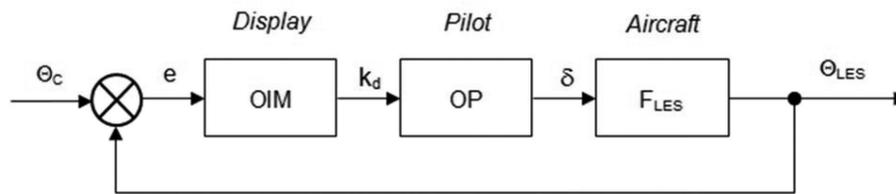
Figure 2 Block diagram of the transfer function of aircraft movement
