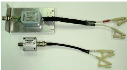
Fig. 5. A photo of Mini-Circuits® FTB-1-6 (down) and North Hills™ 0300BA (up) transformers with cables and electrode clamps
