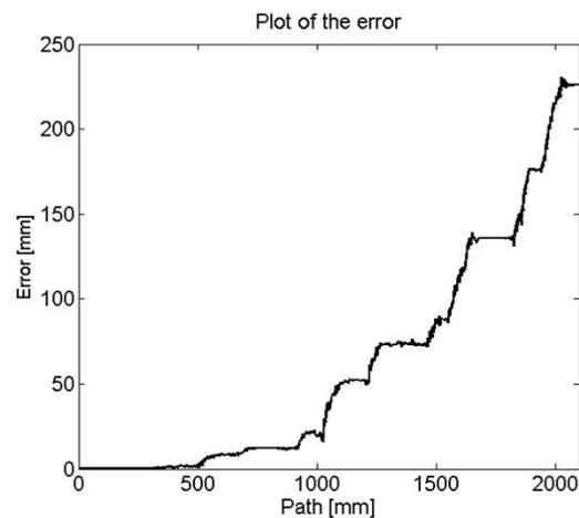
Fig. 16. Open loop test two position error
