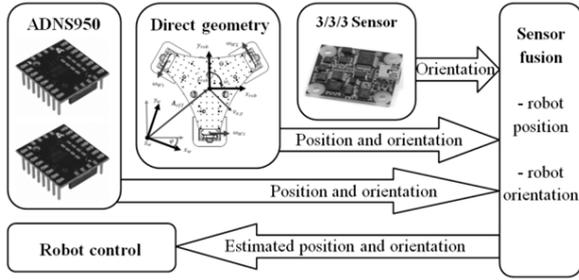
Fig. 3. The sensors on the robot base
