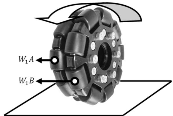
Fig. 2. Contact points of an omni wheel
