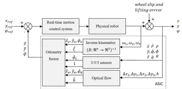
Fig. 12. System block diagram
