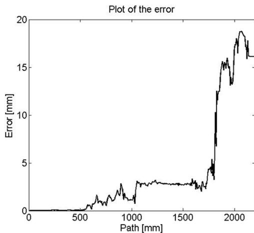
Fig. 14. Open loop test one position error
