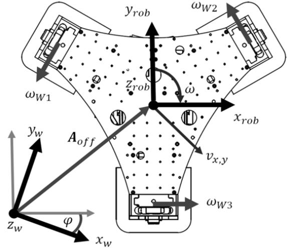
Fig. 4. Robot kinematics
