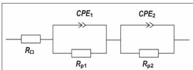
**Figure 3** Equivalent electrical circuit for as-cast and laser hardened AlZn10Si8Mg alloy
