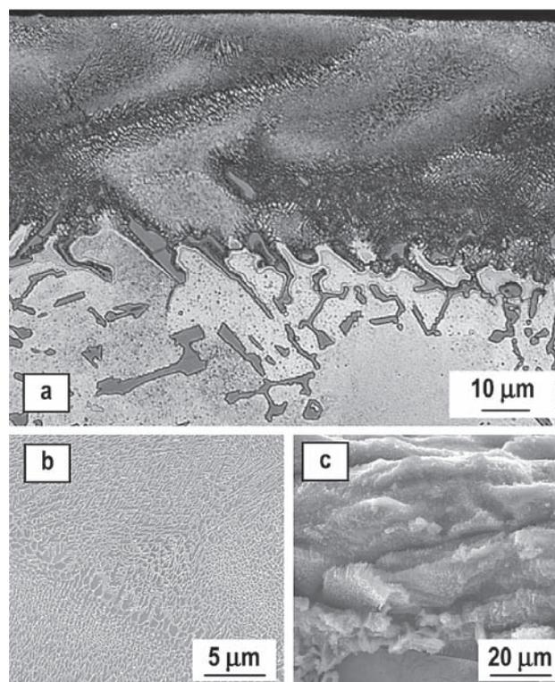
**Figure 2** Microstructure of AlZn10Si8Mg cast alloy, laser layer, etch. Weck-Al
