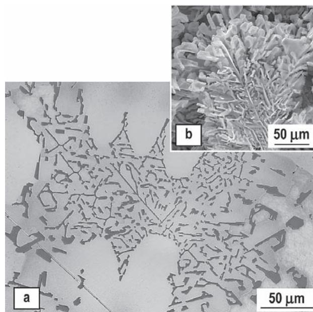
**Figure 1** Microstructure of AlZn10Si8Mg cast alloy, as-cast state, etch. 0,5 % HF
