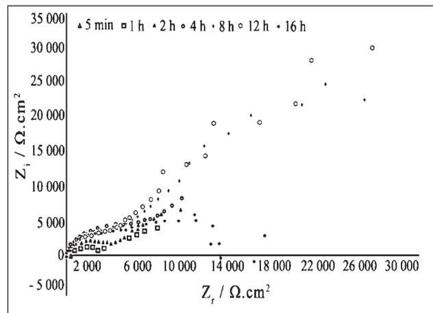
**Figure 4** Nyquist plots for AlZn10Si8Mg alloy (as-cast state) in 1 M NaCl solution
