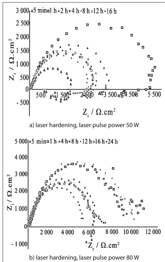
**Figure 5** Nyquist plots for AlZn10Si8Mg samples in 1 M NaCl solution
