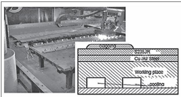
**Figure 1** The view position for the automatic cladding and schematic view of the work table. [7]
