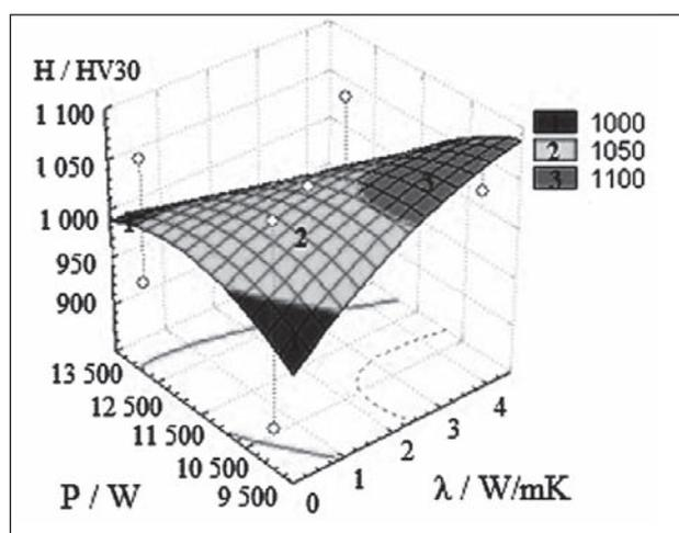
Figure 4 The effects of setting parameters of the power source and the thermal conductivity of the hardness
