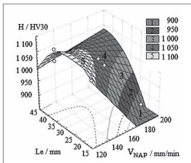
Figure 3 Flow parameters of free outlet electrode of welding speed and hardness
