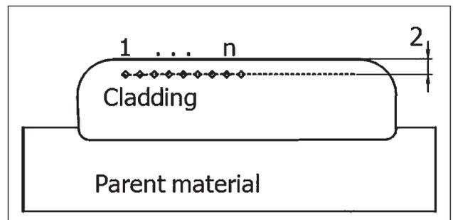
**Figure 2** View of choice of places to measure the hardness, and view of test specimen
