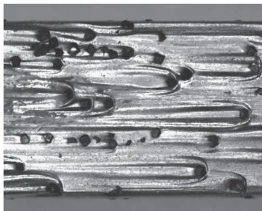
Figure 4 Diamond crystals retained on the cutting surface of a segment
