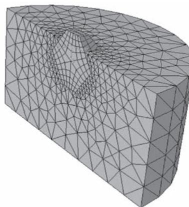
Figure 7 Model of a diamond crystal protruding above the matrix surface
