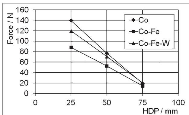
**Figure 9** Tangential force pulling a diamond crystal out of the matrices
