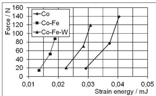
**Figure 10** Pulling force (tangent to the surface) vs. elastic strain energy of the diamond in the matrices
