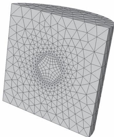
Figure 6 Model of a diamond crystal inside the matrix
