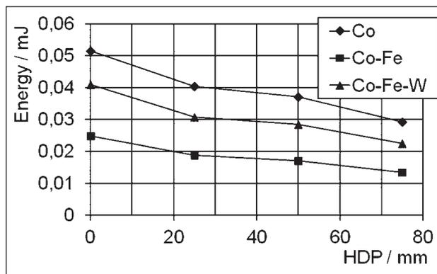
Figure 8 Total strain energy of diamond as a function of the height of diamond protrusion
