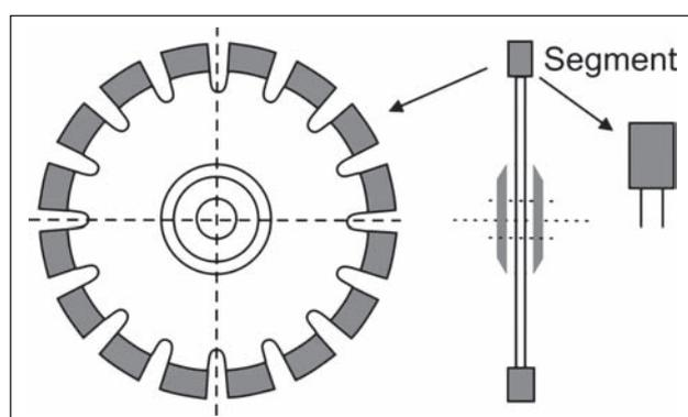
**Figure 1** Schematic representation of a segmental circular saw blade
