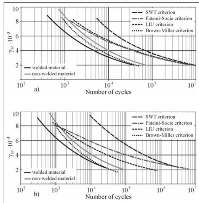
**Figure 8** Comparison of the  $\gamma$ - $N_f$  curves
