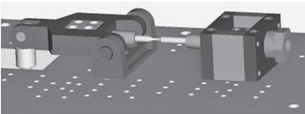
Figure 2 Load system for the bending-torsion load cycle
