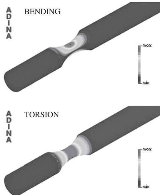
Figure 3 Distribution of equivalent von Mises stress
