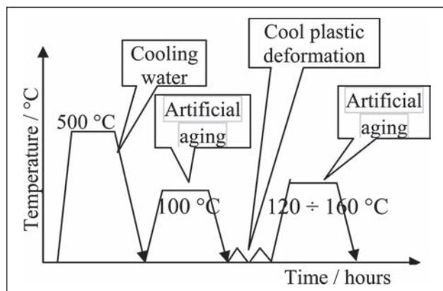
Figure 1 Schematic representation of thermo mechanical processing
