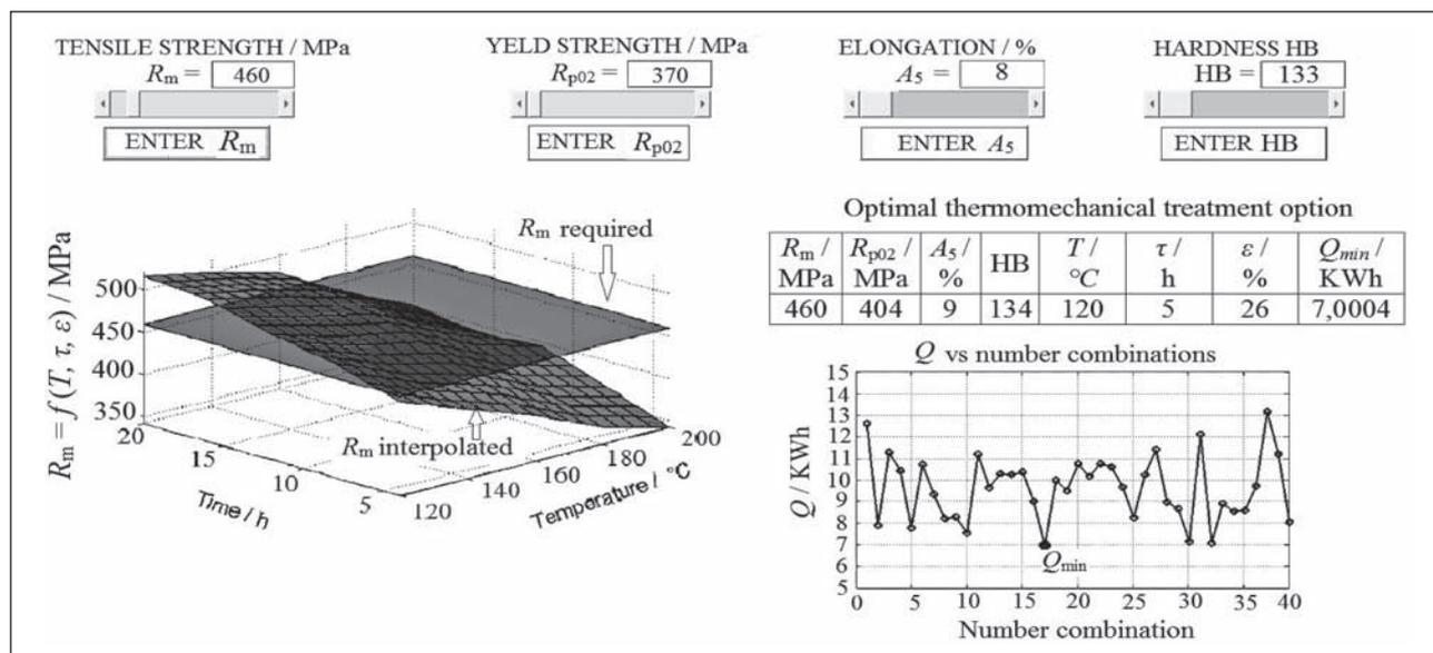
Figure 2 Values of thermo mechanical treatment parameters to achieve  $R_m = 460$  MPa
